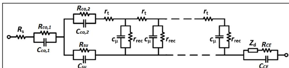
Fig.5. Equivalent circuit model of dye-sensitized solar cell
