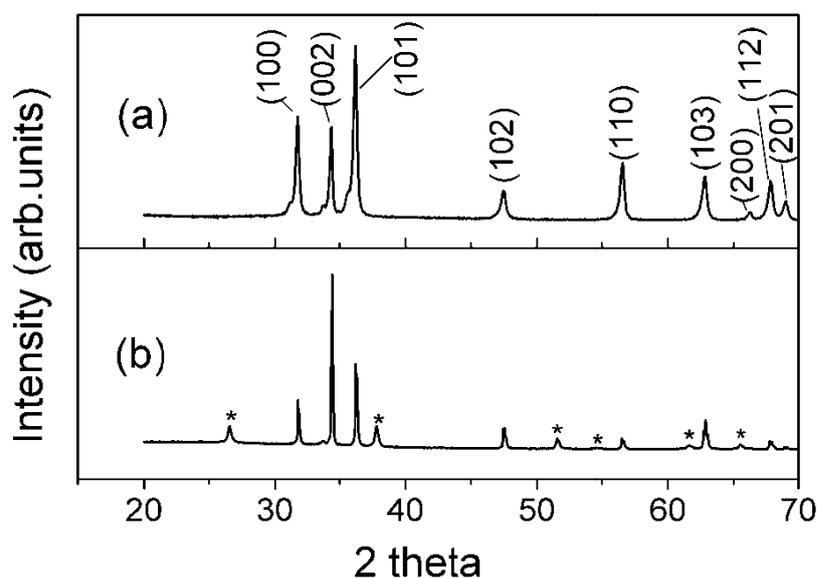
Fig.2. XRD patterns of ZnO (a) nanopowder for electrophoretic deposition treated at 450°C for 30min and (b) nanorod array grown on the FTO electrode. The peaks of the FTO coated glass substrate is indicated by “\*”.
