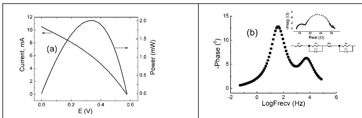
Fig.4. Evaluation of solar cell based on nanostructured ZnO photoanode sensitized with D149 dye under illumination AM 1.5: a) current-voltage characteristics and power profile b) Bode phase representation. The inset shows the equivalent circuit which was fitted the measured spectrum and Nyquist representation of the impedance spectrum.
