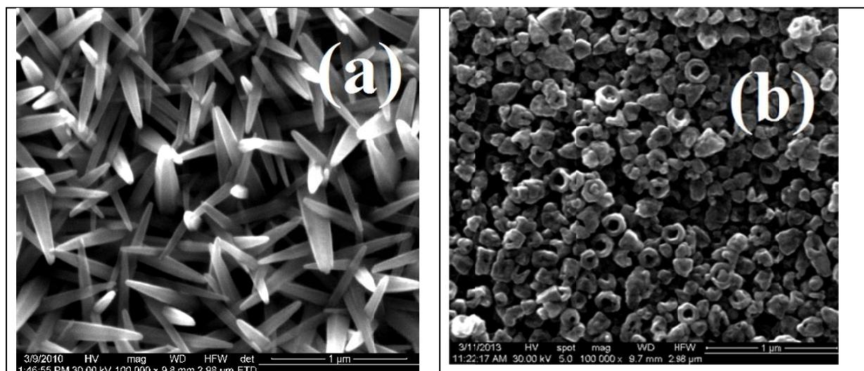
Fig.1. FESEM images of ZnO nanostructures deposited on FTO electrode: a) nanorod array prepared in a hydrothermal-electrochemical process; b) nanopowder for electrophoretic deposition treated at 450°C for 30min.
