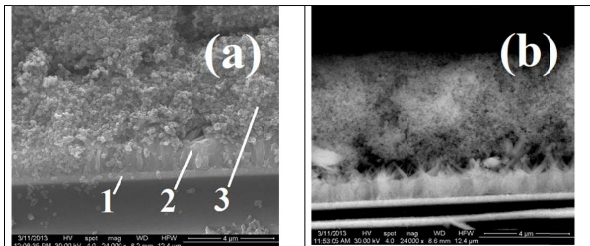
Fig.3. FESEM images of  $\text{ZnO}$  layer structure used for the fabrication of DSC photoanode: (a) 1- $\text{ZnO}$  film; 2- $\text{ZnO}$  nanorod array; 3- $\text{ZnO}$  layer deposited by electrophoretic technique. (b) Imperfect mechanical contact between  $\text{ZnO}$  nanorod array and electrophoretically deposited  $\text{ZnO}$  nanoparticles.
