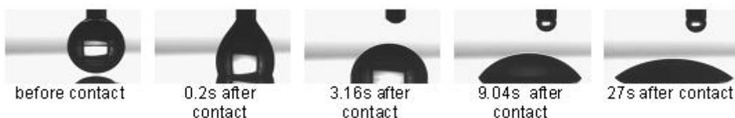
Figure 2: Sequential steps in contact angle determination for AS1 material.
