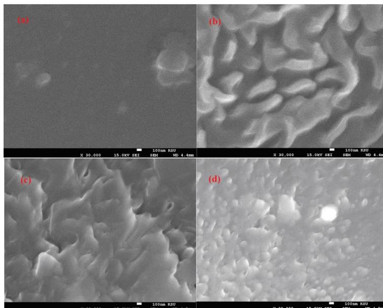
Fig. 3. FESEM morphology of (a) reference, (b)  $1 \times 10^{13}$ , (c)  $1 \times 10^{14}$  and (d)  $1 \times 10^{15}$  ions/cm<sup>2</sup> proton irradiated PM-355 SSNTDs
