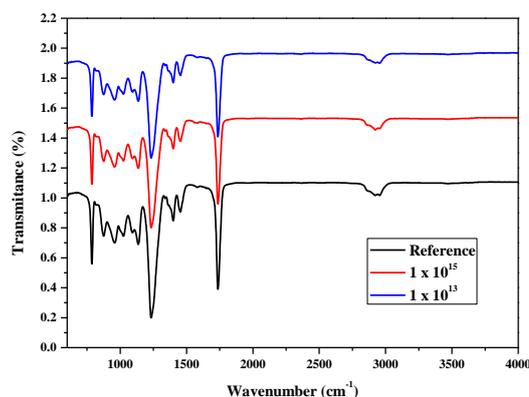
Fig. 2. FTIR spectra of reference and proton irradiated PM-355 SSNTDs
