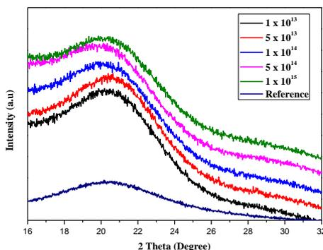
Fig. 1. XRD spectra of PM-355 SSNTDs with and without proton irradiation
