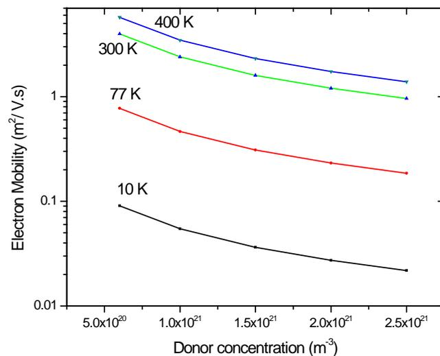
Fig. 3 Drift mobility variation with donor impurity concentration at selected temperatures.
