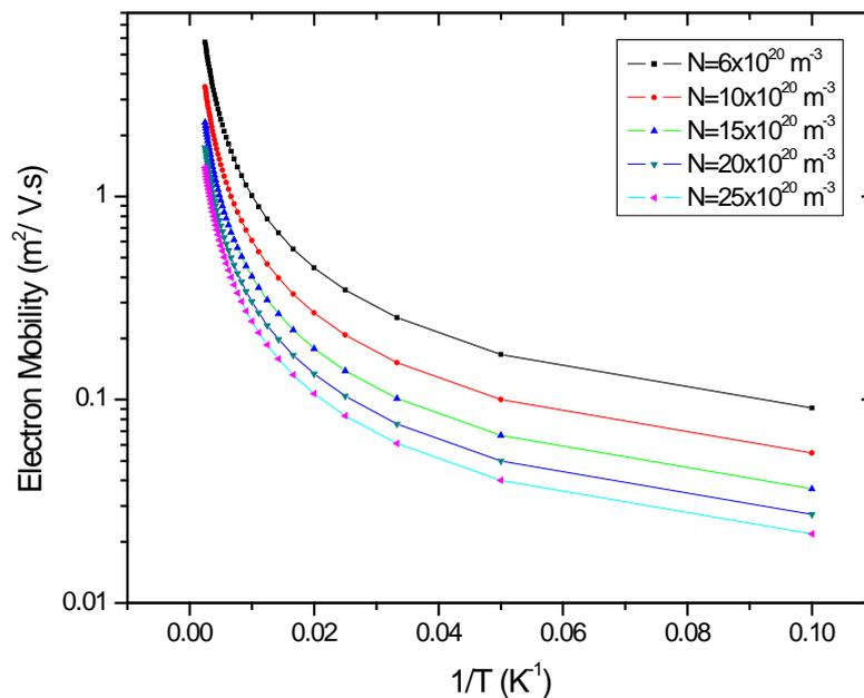
Fig. 2 The electron drift mobility versus inverse of temperature at different donor concentrations.
