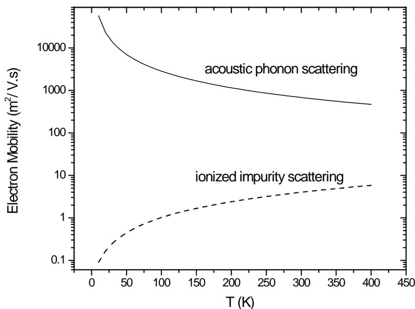
Fig. 1 Mobility versus temperature due to ionized impurities and acoustic phonon scatterings.
