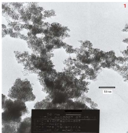
Fig 2. Transmission Electron Micrograph of  $Ni_{0.7}Zn_{0.3}Fe_2O_4$  calcined at 30 °C
