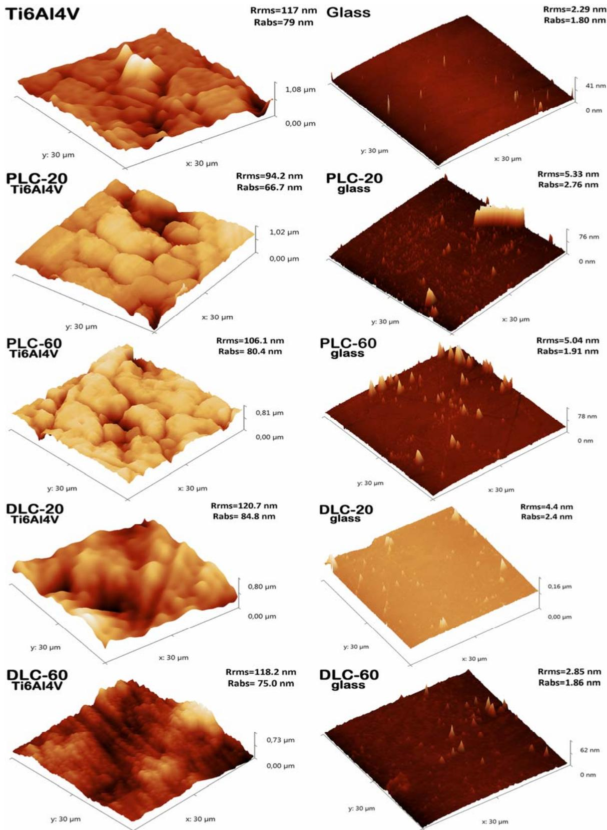
Fig. 4. AFM 3D topographic images for: (a) Ti6Al4V substrate; (b,c) PLC coatings and (d,e) DLC coatings.
