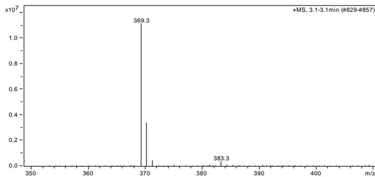
Fig. 3b The full-scan spectrum of cholesterol on the basis the chromatogram from Fig. 3a was built
