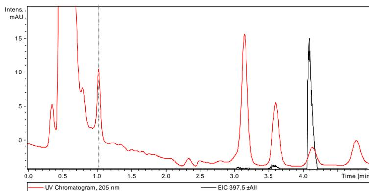
Fig. 5a Chromatogram of the specific ion for sitosterol with  $m/z$  397 (black) and UV chromatogram at 205 nm (red). Retention time for  $\beta$ -sitosterol was 4.1 min.
