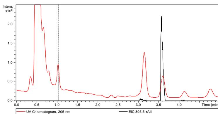
Fig. 4a Chromatogram of the specific ion for stigmasterol with  $m/z$  395 (black) and UV chromatogram at 205 nm (red). Retention time for stigmasterol was 3.6 min.
