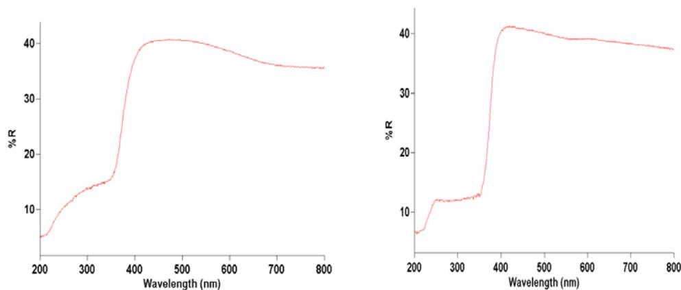
*Fig. 3 The reflectance spectra of ZnO*
