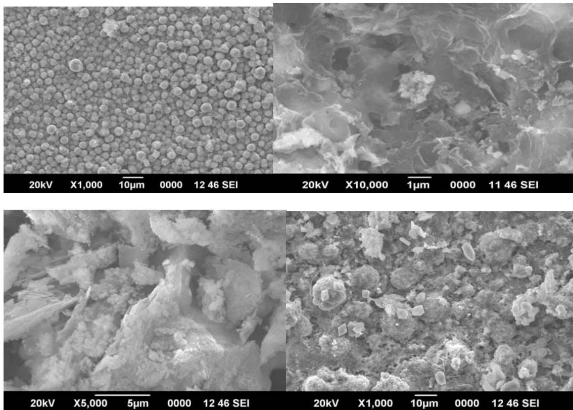
*Fig. 2. SEM images of ZnO film prepared different current densities*
