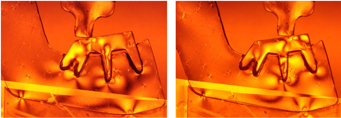
Fig. 5. Model with 3 abutment teeth, strain focused at the level of the intermediate part of the bridge body (between the distal or mesial abutment and the intermediate abutment).
