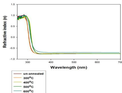
Fig. 6. The refractive index ( $n$ ) of  $\text{TiO}_2$  thin films as a function of wavelength  $\lambda$  at different annealing temperatures.
