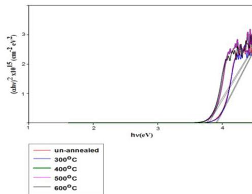
Fig. 5. Plot of  $(\alpha h\nu)^2$  vs  $h\nu$  for TiO<sub>2</sub> thin films with different annealing temperatures.
