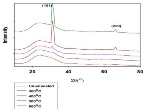
Fig. 1. X-Ray patterns of un-annealed TiO<sub>2</sub> thin films at different annealing temperatures (a) un-annealed (b) 300°C (c) 400°C (d) 500°C and (e) 600°C.
