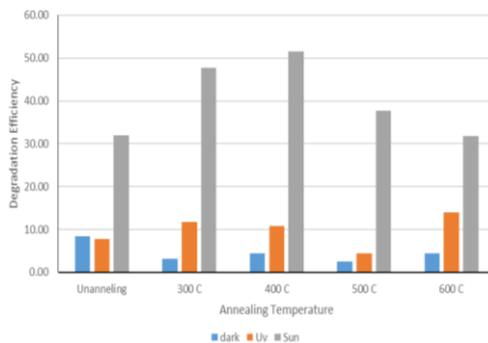
Fig. 7. Degradation efficiency of thin films at different annealing temperatures under UV light and Sun light.
