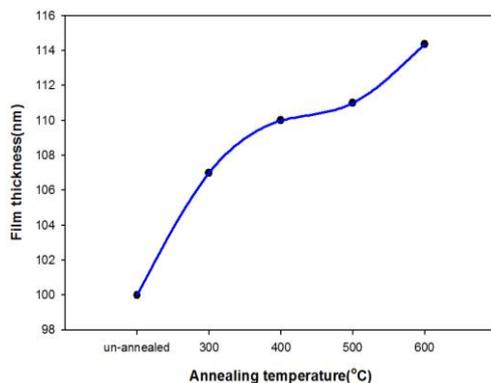
Fig. 2. The variation of the films thickness of  $\text{TiO}_2$  thin films with annealing temperatures.
