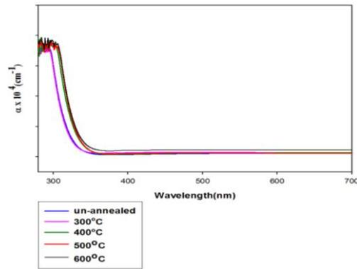
Fig. 4. Absorbance spectra of TiO<sub>2</sub> films at different annealing temperature.
