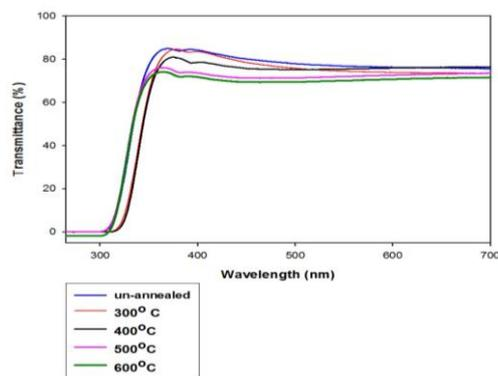
Fig. 3. Optical Transmission spectra of  $\text{TiO}_2$  films at different annealing temperatures.
