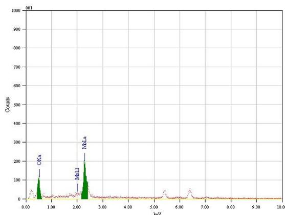
Fig. 4: EDAX pattern of  $\text{MoO}_3$  films electrodeposited at pH 2 and at  $550^\circ\text{C}$ .
