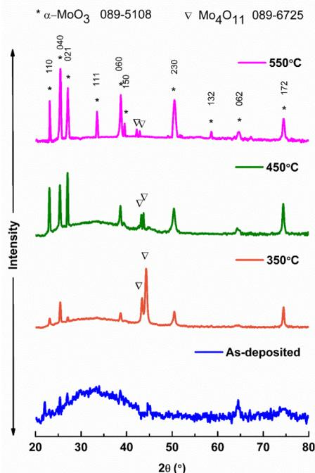
Fig. 2: XRD pattern of  $\text{MoO}_3$  films electrodeposited at pH 2 and at different temperatures (a) as-deposited, (b) 350°C, (c) 450°C, and (d) 550°C
