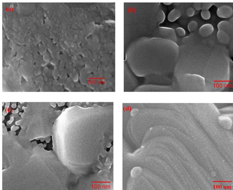
Fig. 3: Electron micrographs of  $\text{MoO}_3$  films electrodeposited at pH 2 and at different temperatures (a) as-deposited, (b)  $350^\circ\text{C}$ , (c)  $450^\circ\text{C}$ , and (d)  $550^\circ\text{C}$
