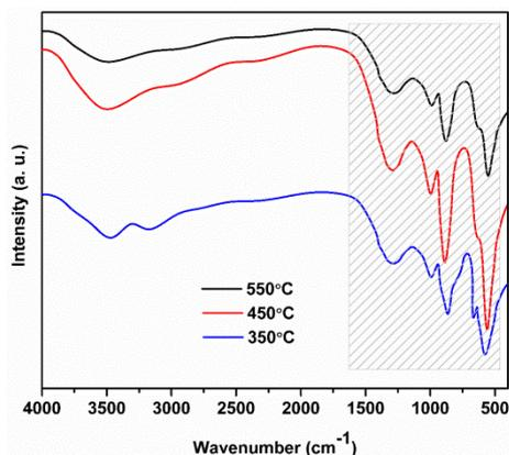
Fig. 5: FTIR of  $\text{MoO}_3$  films electrodeposited at pH 2 and at different temperatures (a) as-deposited, (b) 350°C, (c) 450°C, and (d) 550°C
