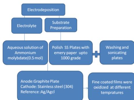
Fig. 1. Schematic representation of synthetic procedures for the molybdenum trioxide thin films by electrodeposition method
