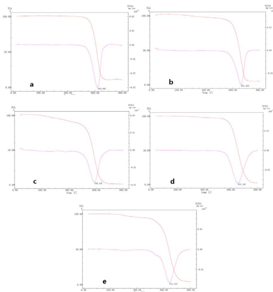
Fig. 4 Thermogravimetric curve of SWCNTs
