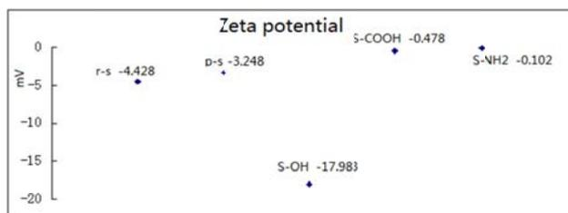
Fig. 2 Zeta potential of SWCNTs (pH 7.0)
