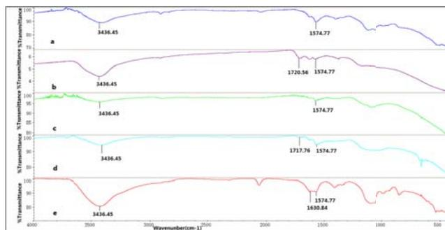
Fig.1 FTIR spectra of SWCNTs modified by chemical groups Note: a: raw-SWCNTs (r-S), b: purified SWCNTs (p-S), c: SWCNTs-OH (S-OH), d: SWCNTs-COOH (S-COOH), e: SWCNTs-NH<sub>2</sub> (S-NH<sub>2</sub>)
