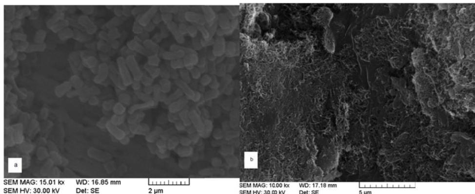
Fig.6 Scanning electron microscopy images of *E. coli* cells (a) without SWCNTs (b) with SWCNTs
