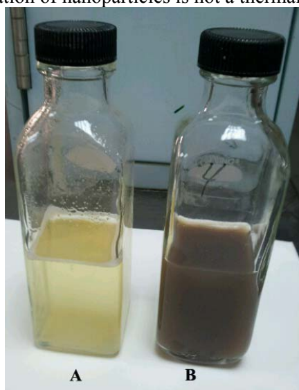
Fig. 1. Conical flasks containing the Fusarium semitectum KSU-4 filtrate in an aqueous solution of 10^{-3} \text{ M AgNO}_3 at the beginning of the reaction (A) and after 3 days of reaction (B).
