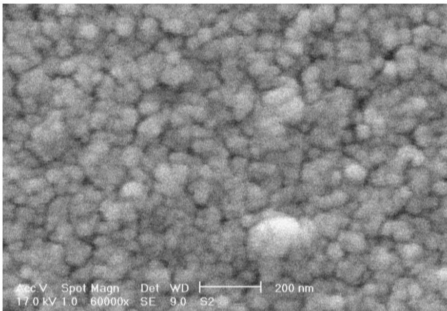
*Fig.3 Top view of SEM image of  $TiO_2$  film coated on FTO glass*
