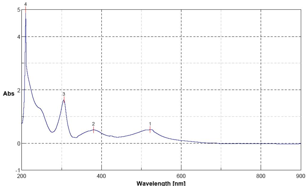
*Fig.5 Spectral response of  $TiO_2$  electrode coated with Ruthenium 535-bisTBA dye*
