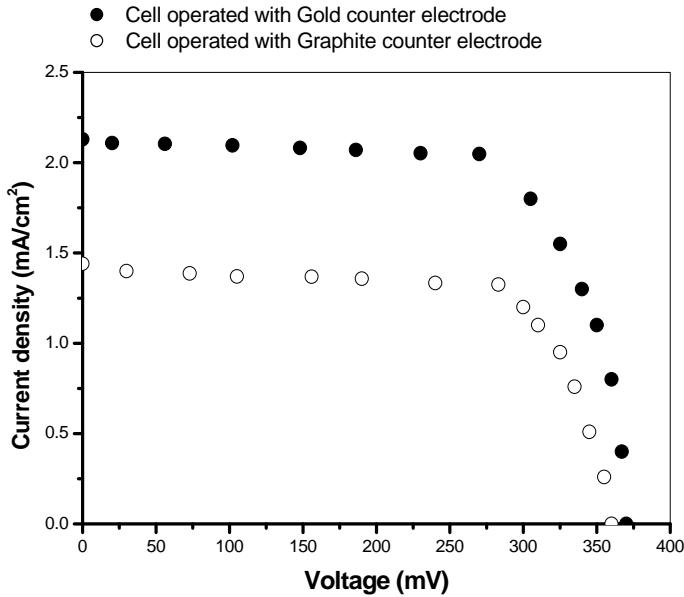
Fig. 6. Photovoltaic response of fabricated DSSCs under illumination.
