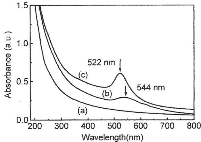
Fig. 3. UV-Vis Spectroscopy of CdS nanoparticles prepared at (a) 500°C (b) 600°C (c) 700 °C.
