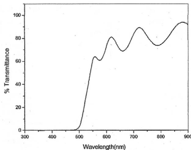
Fig. 4. Optical transmission spectrum of CdS nanoparticles.
