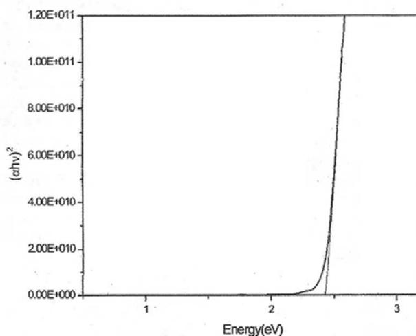
Fig. 5.  $(ahv)^2$  vs  $h\nu$  of CdS nanoparticles.
