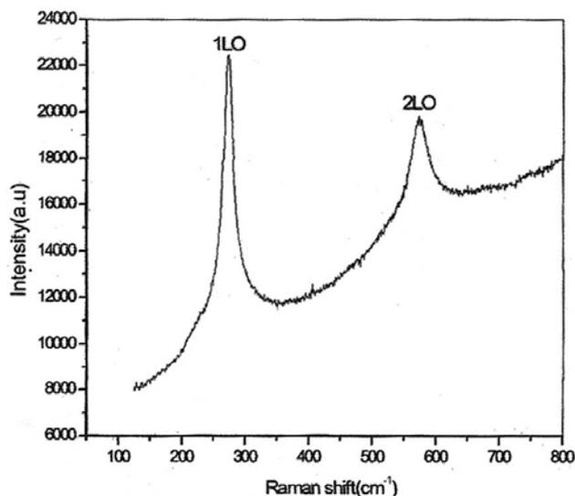
Fig. 6 Raman spectrum of CdS nanoparticles.
