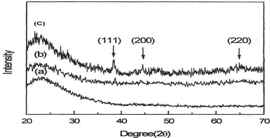
Fig. 1. X-ray diffraction pattern of CdS nanoparticles prepared at (a) 500<sup>0</sup>C (b) 600<sup>0</sup>C (c) 700<sup>0</sup>C
