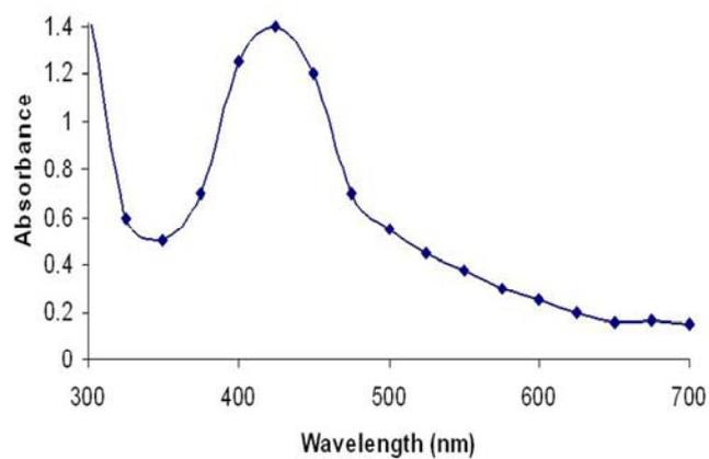
Fig. 2. UV-Vis absorption spectrum of silver nanoparticles synthesized by treating 1mM aqueous  $\text{AgNO}_3$  solution with 10% Papaya fruit extract after 5 hrs.
