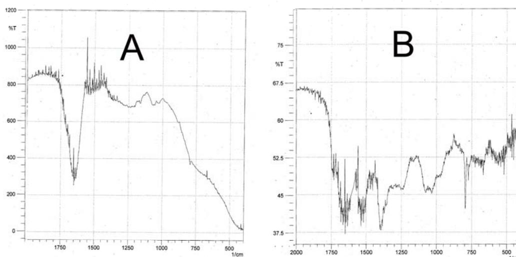
Fig. 5. FTIR spectra of vacuum dried powder of (a) Papaya fruit extract (b) nanoparticles synthesized by 10% fruit extract solution.
