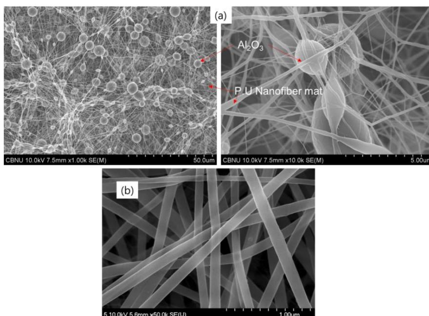
Fig. 3 FE-SEM images of (a)  $\text{PU}/\text{Al}_2\text{O}_3$  composite mat, (b) Pristine PU
