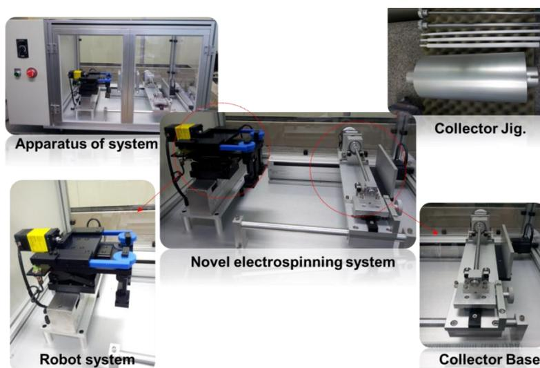
Fig. 1 Schematic of experiment equipment
