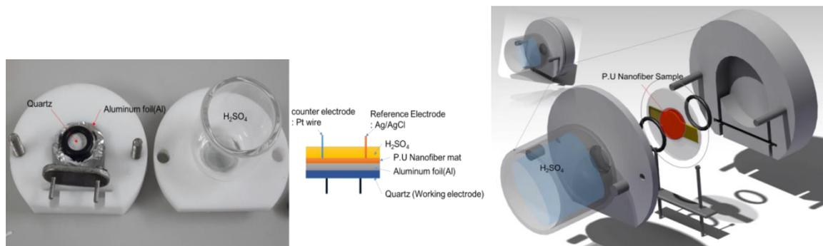
Fig. 2. Real electrochemical experiment configuration using QCM
