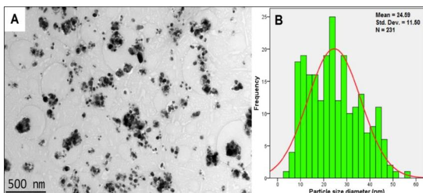
Fig. 4. TEM image of sodium alginate/Ag-NPs after irradiation (A) and its histogram (B).
