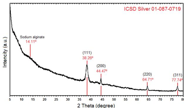
Fig. 5. XRD pattern of synthesized sodium alginate/Ag-NPs after 240 min irradiation.
