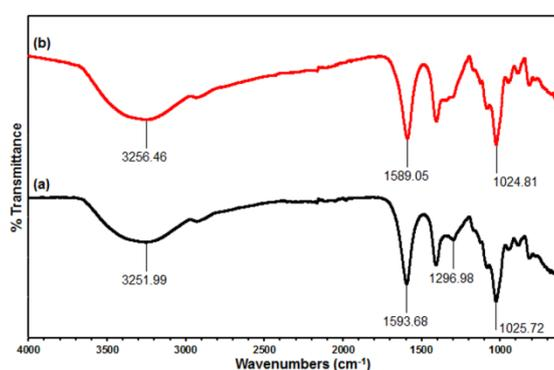
Fig. 6. FT-IR spectra of sodium alginate media (a) and sodium alginate/Ag-NPs 240 min ultrasound irradiation (b)
