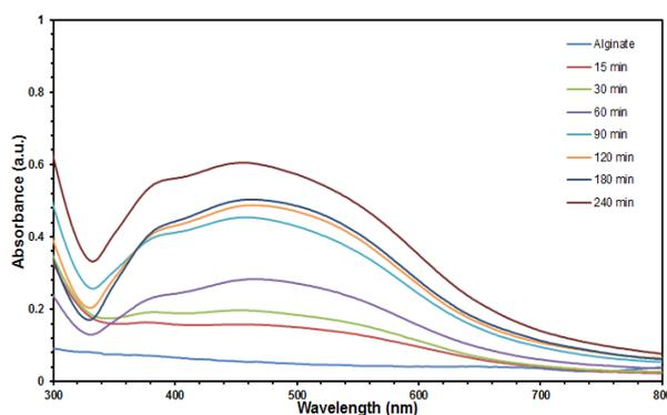
Fig. 2. The UV-Vis absorption spectra of synthesizing Ag-NPs on sodium alginate under varying times of ultrasound irradiation.
