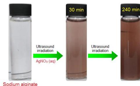
Fig. 1. Photographs of sodium alginate before irradiation and sodium alginate/Ag-NPs after irradiation (30 and 240 min).
