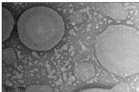
Fig. 3. TEM image of sodium alginate before ultrasound irradiation.
