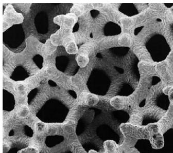
*Fig. 2. Trabecular Metal (TM). An image made by scanning electron microscopy demonstrates highly porous microstructure.*
