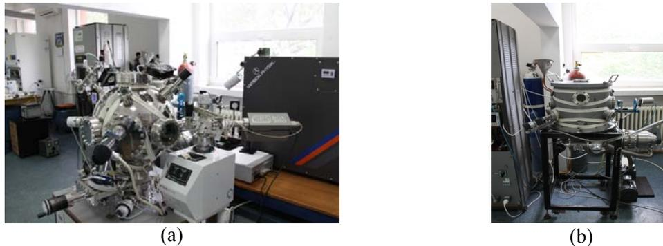
Fig. 3. Deposition (a) and (b) stainless steel reaction chambers [14].
