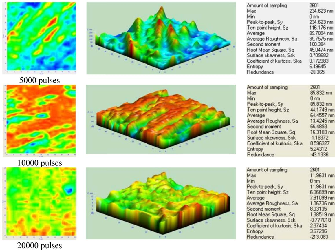
Fig. 5. Roughness of 316L stainless steel substrate coated with TiN layer measured using NTEGRA Atomic force Microscope.
