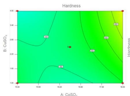
Fig. 3. The contour map of microhardness response surface.
