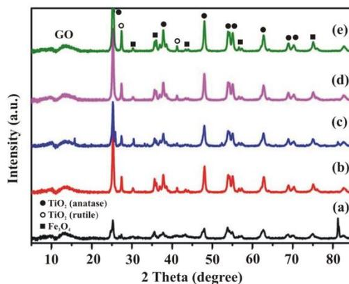
Fig. 4. XRD patterns as-prepared GF: $\text{TiO}_2$  nanocomposites with weight ratio of (a) 1:3; (b) 1:4; (c) 1:5; (d) 1:6 and (e) 1:7.
