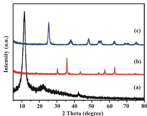
Fig. 3. XRD patterns of (a) GO, (b)  $\text{Fe}_3\text{O}_4$  and (c)  $\text{TiO}_2$ .
