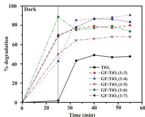
Fig. 7. Photocatalytic degradation efficiency of MB under visible light utilising  $\text{TiO}_2$  and as-prepared GF: $\text{TiO}_2$  nanocomposites.
