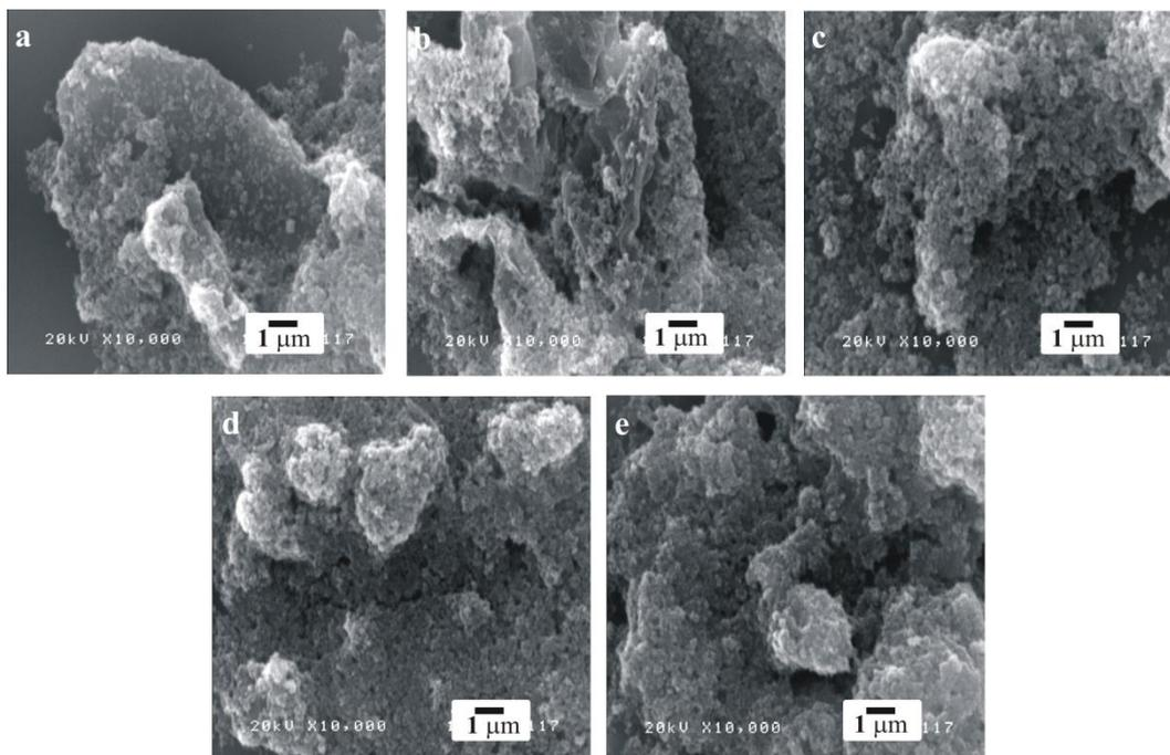
Fig. 1. SEM images of as-prepared GF:TiO<sub>2</sub> nanocomposites with weight ratio (a) 1:3, (b) 1:4, (c) 1:5, (d) 1:6 and (e) 1:7.
