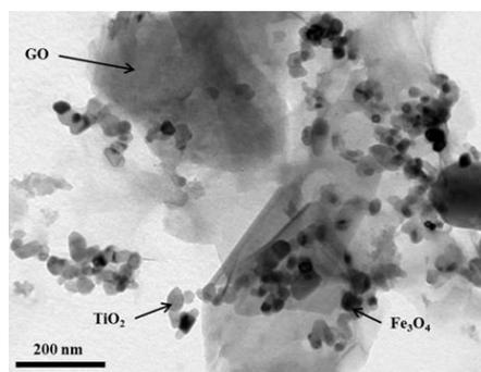
Fig. 2. TEM image of as-prepared GF:TiO<sub>2</sub> nanocomposites with weight ratio 1:5.
