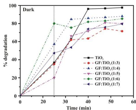
Fig. 6. Photocatalytic degradation efficiency of MB under UV light utilising  $\text{TiO}_2$  and as-prepared GF: $\text{TiO}_2$  nanocomposites.
