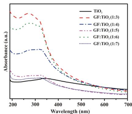
Fig. 5. UV-vis spectra of  $\text{TiO}_2$  and as-prepared GF: $\text{TiO}_2$  nanocomposites with weight ratio of 1:3, 1:4, 1:5, 1:6 and 1:7.
