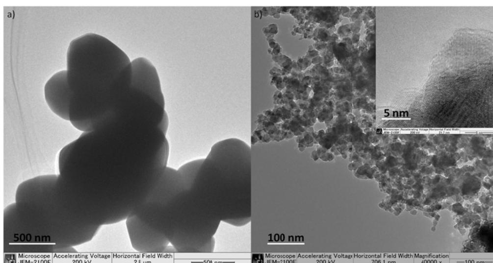
*Fig. 8 TEM images of (a) commercial ZnO powder, and (b) ZnO NPs fabricated by PLA.*
