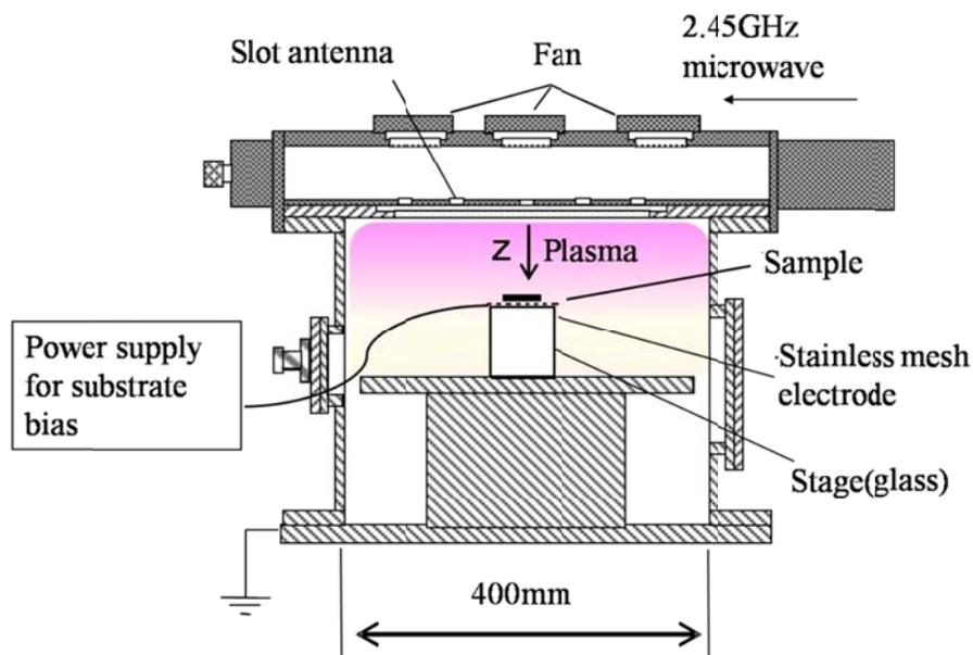
Fig. 2 Schematic drawing of the surface wave plasma device.
