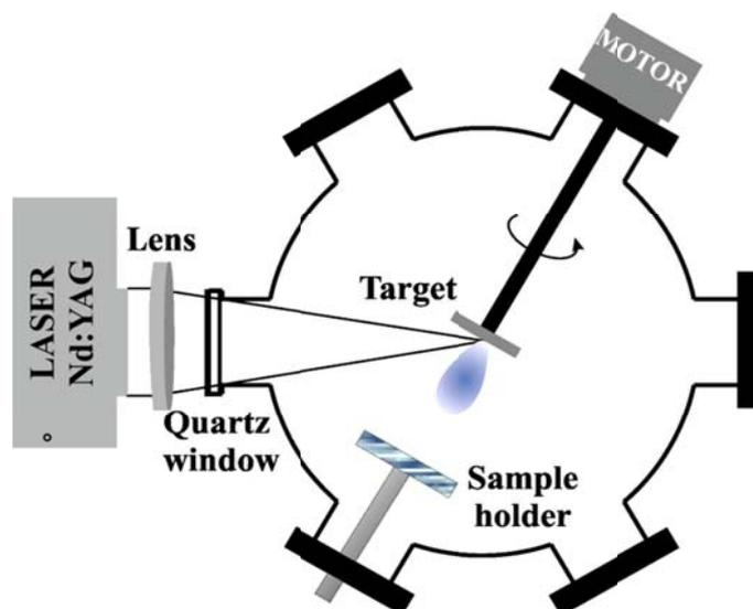
Fig. 3 Schematic representation of the Nd:YAG PLA experimental setup.
