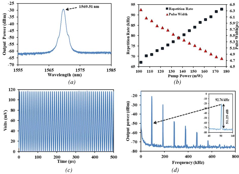
Fig. 3. Q-switching results (a) Output spectrum (b) repetition rates and pulse widths versus pump power (c) typical pulse train (d) RF spectrum
