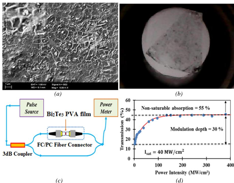
Fig. 1.  $\text{Bi}_2\text{Te}_3$  characteristics (a) image of the SA film onto the fiber ferrule (b) FESEM image (c) the balance twin-detector measurement set up (d) nonlinear transmission curve.
