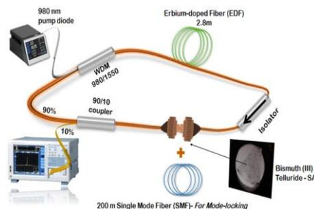
Fig. 2. The proposed Q-switched EDFL cavity with  $\text{Bi}_2\text{Te}_3$  PVA film as a SA. The mode-locked pulses were generated with the addition of 200 m long SMF.
