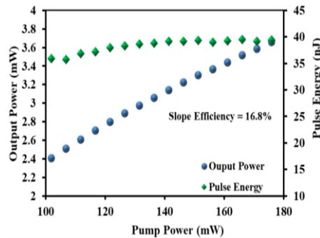
Fig. 4. Output power and pulse energy at various pump powers.
