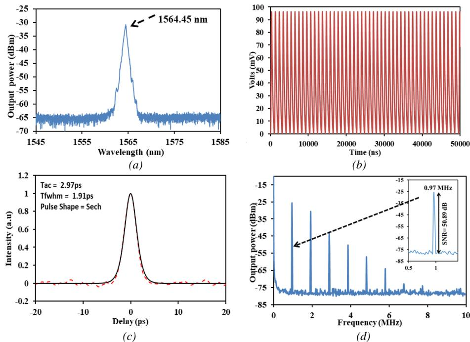
Fig. 5. Mode-locking performances (a) output spectrum with Kelly sidebands (b) typical pulse train (c) autocorrelator trace (d) RF spectrum
