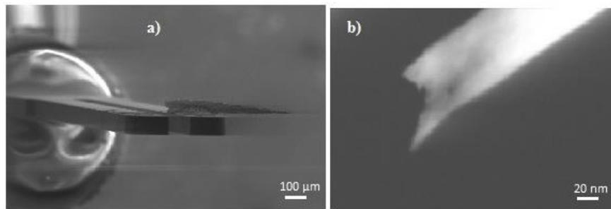
Fig. 2.: a) The etched Platinum-Rhodium wire's SEM image that is attached to one electrode of the tuning fork. b) The sharpness of the tip's vertex in a high-magnification image.
