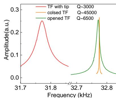
Fig. 3: The tuning fork's frequency spectrum in an evacuated closed case (yellow), opened in air (green), and after attaching the tip to the TF (red).
