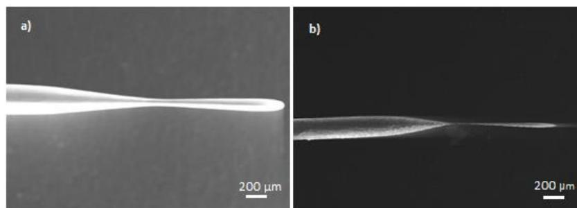
*Fig. 1. A sequence of tip images taken by SEM at different steps of the electrochemical etching procedure. a) A typical droplet shape with a thick neck after the first etching step. b) The final tip shape after polishing in sulfuric acid.*
