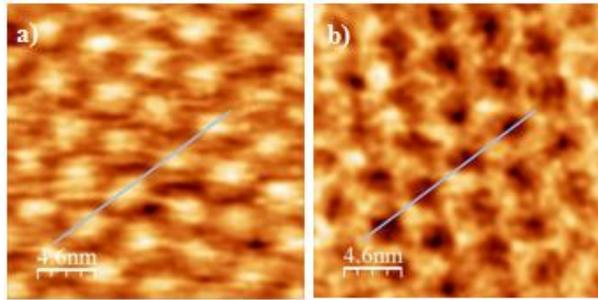
Fig. 4: STM/AFM measurements of moiré pattern on HOPG surface. a) Constant-current STM topography. b) Simultaneously measured frequency shift
