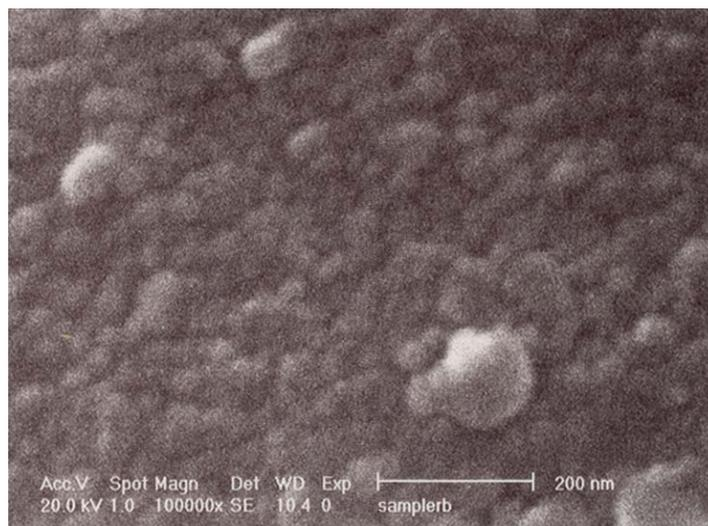
*Fig. 8 SEM photographs of Ag / TiO<sub>2</sub> nano particles on Ti sheet by electrochemical method.*
