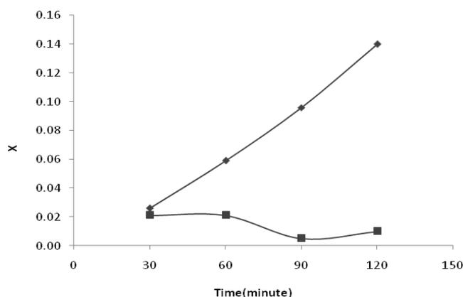
Fig. 5 Effect of O<sub>2</sub> in photodegradation of MO with Ag / TiO<sub>2</sub> nano particles in pH=2, λ=510 nm, MO concentration 6.3×10<sup>-3</sup> M and 150 min irradiation. (■) Absence O<sub>2</sub>. (◆) present O<sub>2</sub>.
