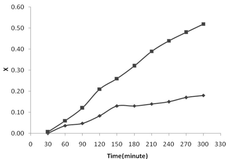
Fig. 1 Comparison of the photocatalytic degradation of MO under UV light with ( $\blacklozenge$ )  $\text{TiO}_2$  and ( $\blacksquare$ )  $\text{Ag} / \text{TiO}_2$  nano particles. Experimental condition: MO concentration  $6.3 \times 10^{-3}$  M, pH = 2,  $\lambda = 510$  nm, presence  $\text{O}_2$  and 5h irradiation.
