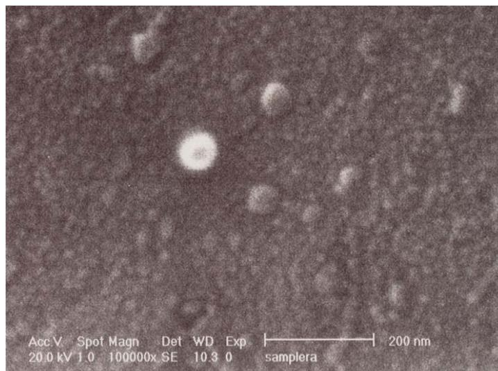
Fig. 7 SEM photographs of TiO<sub>2</sub> nano particles on Ti sheet by electrochemical method.
