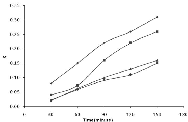
Fig. 4 Effect of distance between light source and Ag / TiO<sub>2</sub> nano particles on the photodegradation of MO with Ag / TiO<sub>2</sub> nanoparticles (■) 51cm, (◆) 56cm, (▲) 61cm, (●) 66cm, Experimental condition: MO concentration  $6.3 \times 10^{-3}$  M, pH = 2,  $\lambda=510$  nm, presence O<sub>2</sub> and 5h irradiation.
