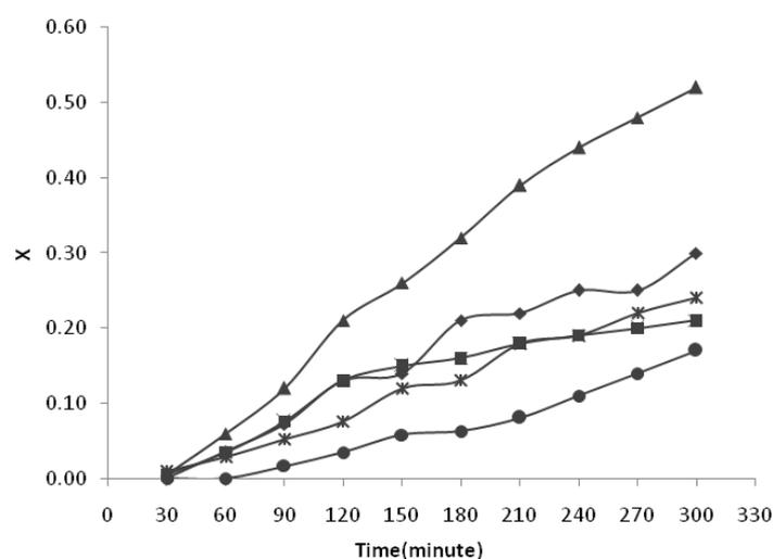
Fig. 2 Effect of Ag concentration on the photo degradation of MO with  $\text{Ag} / \text{TiO}_2$  nano particles, number of immersion ( $\blacklozenge$ ) 10 times, ( $\blacksquare$ ) 30 times, ( $\blacktriangle$ ) 40 times, ( $\bullet$ ) 50 times, ( $\star$ ) 60 times. Experimental condition: MO concentration  $6.1 \times 10^{-5}$  M, pH = 2,  $\lambda = 510$  nm, presence  $\text{O}_2$  and 5h irradiation.
