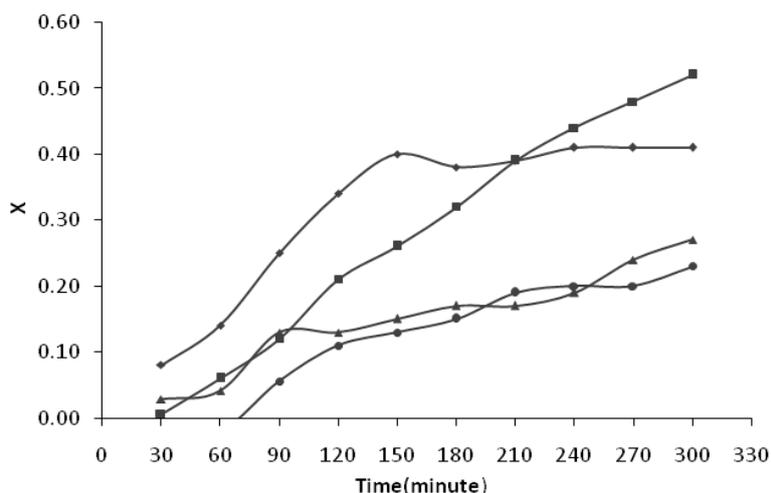
Fig. 3 Photodegradation of MO at various concentration of MO with Ag / TiO<sub>2</sub> nanoparticles in pH=2,  $\lambda=510$  nm, presence O<sub>2</sub>, and 5h irradiation. (■)  $6.1 \times 10^{-5}$ , (▲)  $4 \times 10^{-5}$ , (◆)  $2 \times 10^{-5}$ , (●)  $1 \times 10^{-5}$
