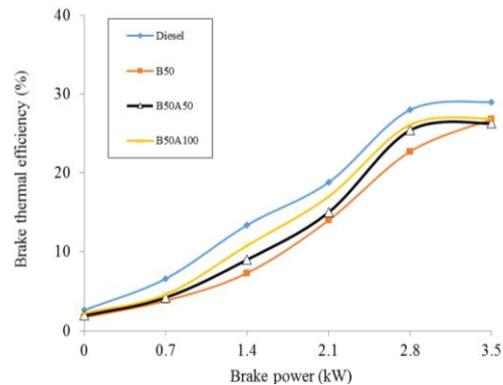
Fig. 6. Variation of BTE for tested fuels with different load conditions.
