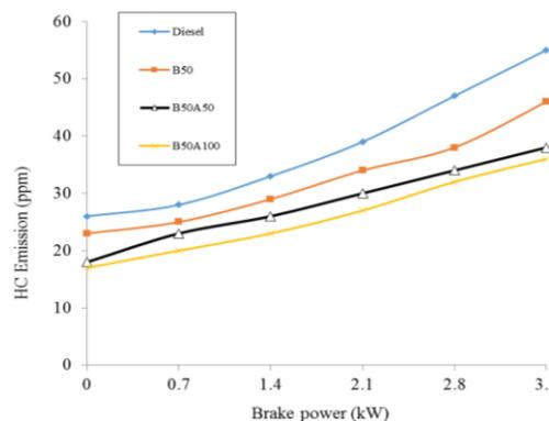
Fig. 3. Variation of HC emissions for tested fuels with different load conditions.
