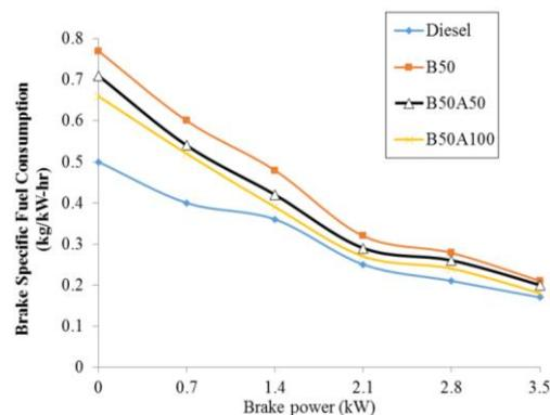
Fig. 7. Variation of BSFC for tested fuels with different load conditions.
