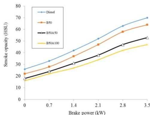
Fig. 5. Variation of smoke opacity for tested fuels with different load conditions.
