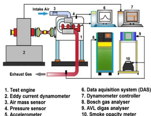
Fig. 1. Experimental setup layout
