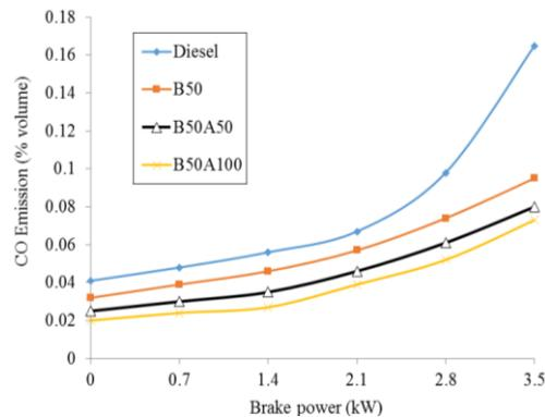
Fig. 2. Variation of CO emissions for tested fuels with different load conditions.
