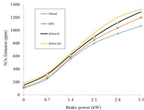
Fig. 4. Variation of  $\text{NO}_x$  emissions for tested fuels with different load conditions.
