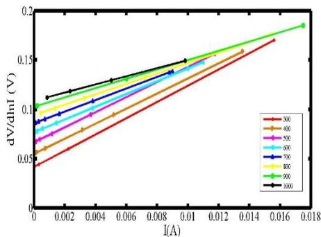
Fig. 2.  $\frac{dV}{d\ln I}$  vs current curve of the ZnO fabricated Schottky diode.
