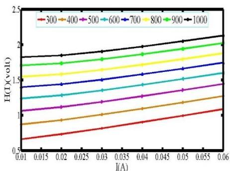
Fig. 3. Cheung function as a function of current I.
