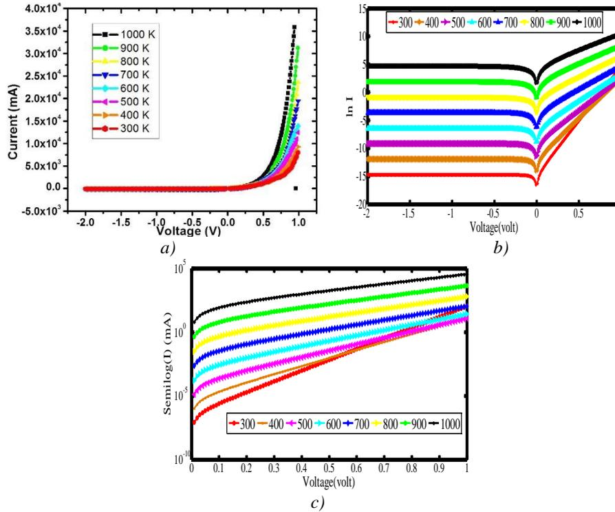
Fig. 1. Current-Voltage characteristics of Schottky diode in the temperature range of 300K-1000K: (a) I-V(b)  $\ln I$ -V (c) Semilog I-V.
