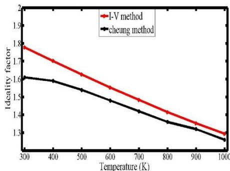
Fig. 5. Ideality factors as a function of temperature.
