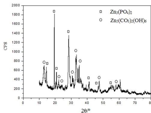
Fig. 1 The XRD pattern of precipitations obtained by microbial method
