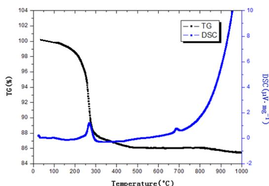
Fig. 5 Thermal analysis curves of precipitations obtained by microbial method
