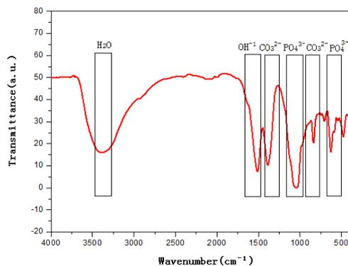
Fig. 4 FTIR spectra of precipitates obtained by microbial method
