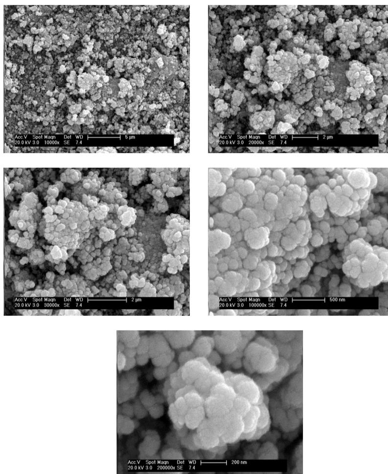
Fig. 3 Different magnification of SEM images of precipitations obtained by microbial method
