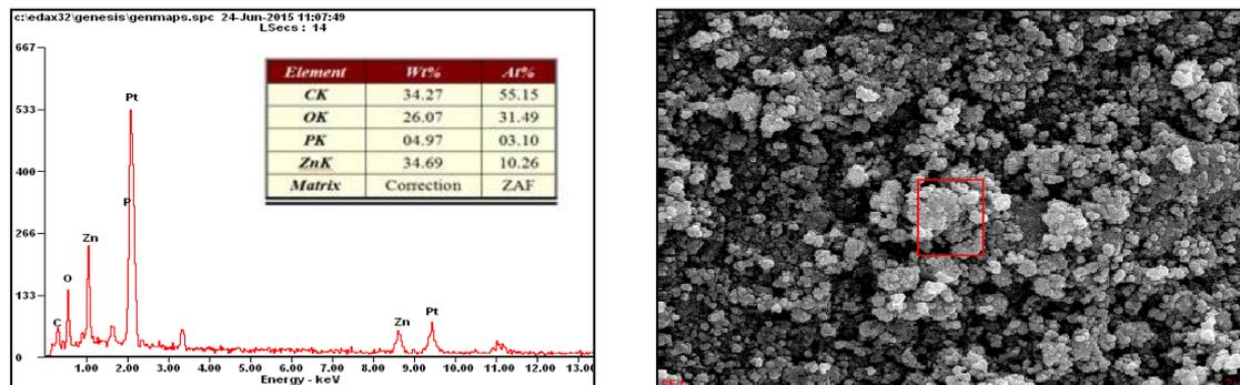
Fig. 2 EDS spectrum of precipitations obtained microbial method
