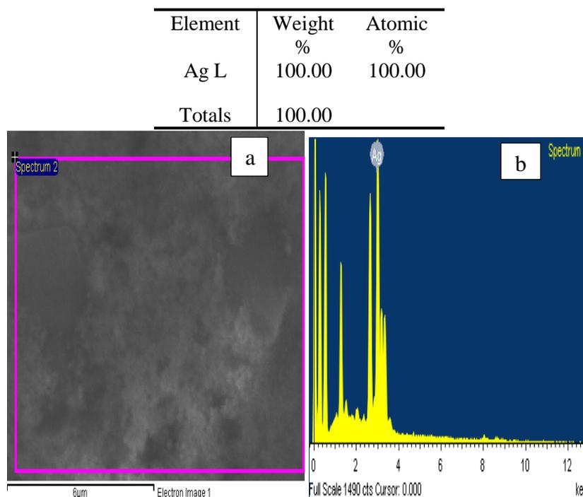
Fig.2. (a) SEM image, (b) EDS pattern of spherical AgNPs prepared.
