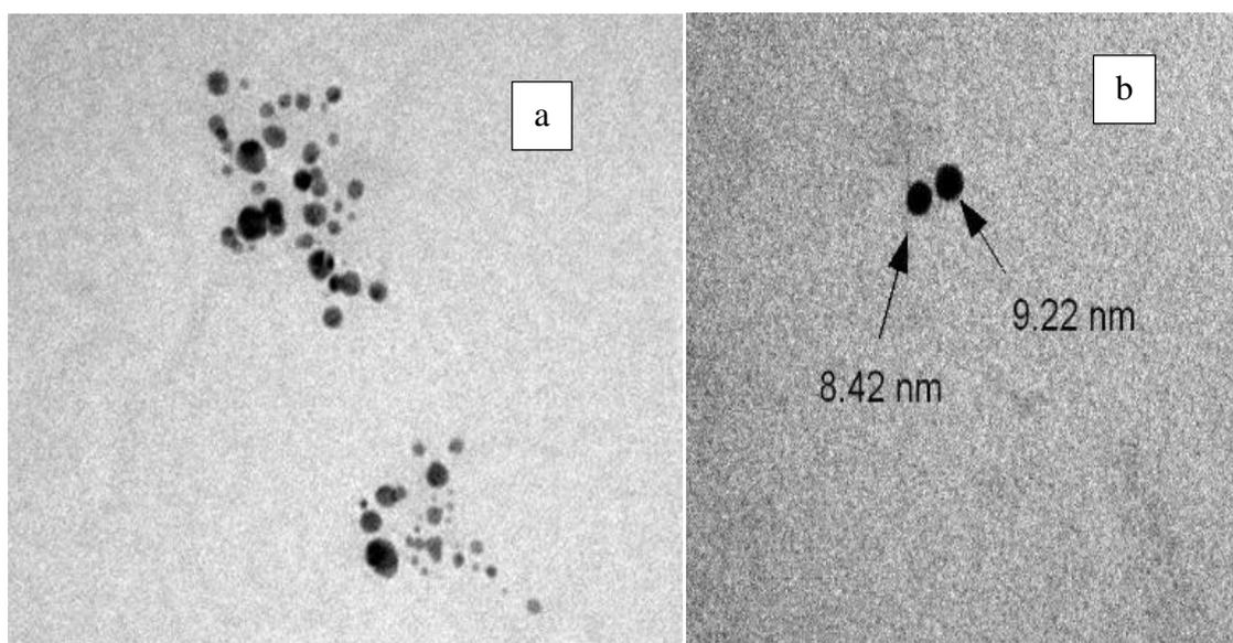
*Fig. (1).TEM image of spherical silver nanoparticles*
