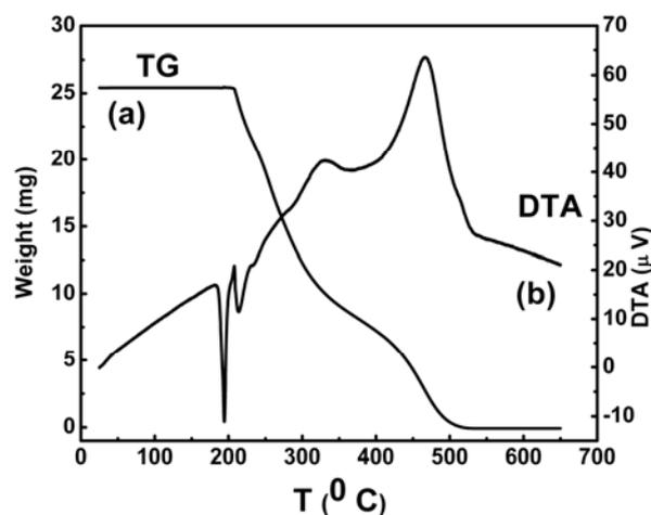
Fig. 2. The DTA/TGA evolution curves for sucrose powder.
