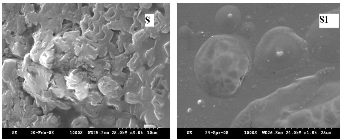
Fig. 1. The SEM images of sucrose powder (sample S) and thin films (sample S1).
