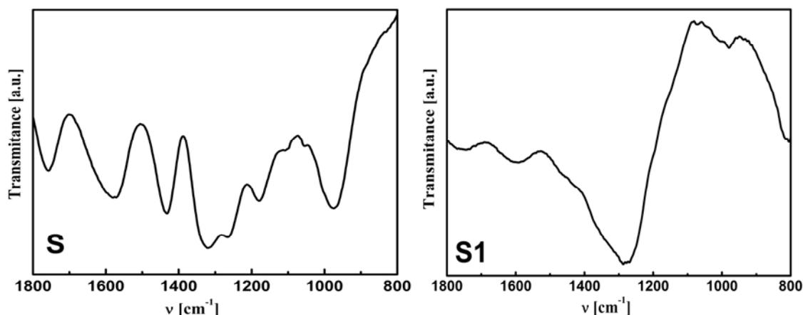
Fig. 3. The FT-IR spectra of sucrose powder (sample S) and thin films (sample S1).
