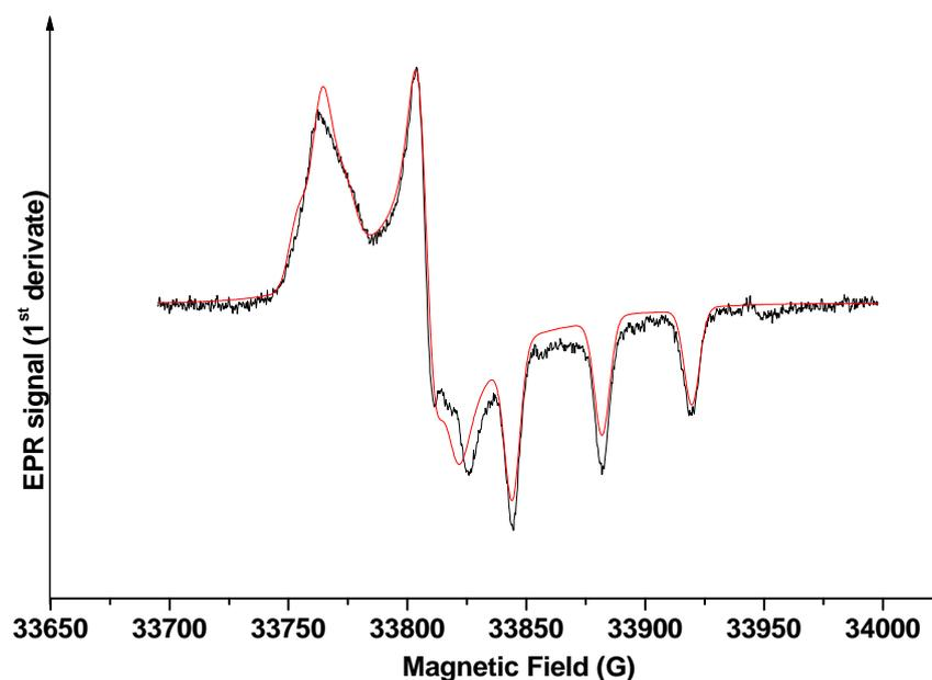
*Fig. 3. Rigid-limit experimental high-field EPR spectrum (continuous lines, first-derivative representation,  $T = 166$  K,  $\nu = 95$  GHz) for methemoglobin. Red line represents the calculated line shape obtained by a modified version of the program DIPFIT (fittings were performed with two sets of  $g_{xx}$  parameters and only one set for  $g_{yy}$ ,  $g_{zz}$  and A-tensor parameters).*
