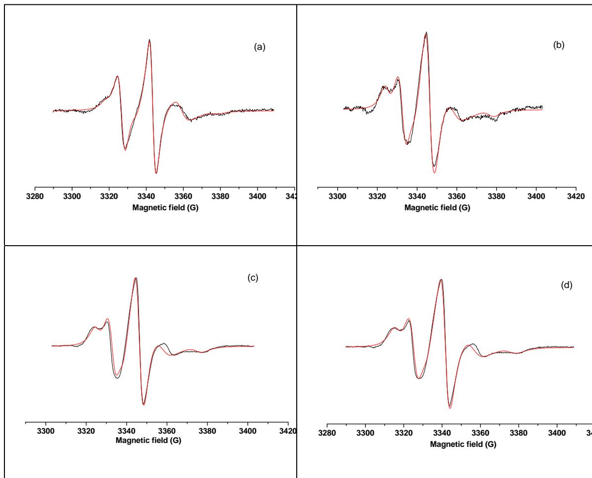
*Fig. 4. X-band EPR spectra of methemoglobin spin-labeled in position  $\beta$ -93\* in solution (a) and in the adsorbed state on bioglass system 1 (b), system 2 (c), and system 3 (d). The red lines represent the best fits of simulated spectra to the experimental ones, using the  $g$  and  $A$ -tensor values determined by W-band EPR spectroscopy.*
