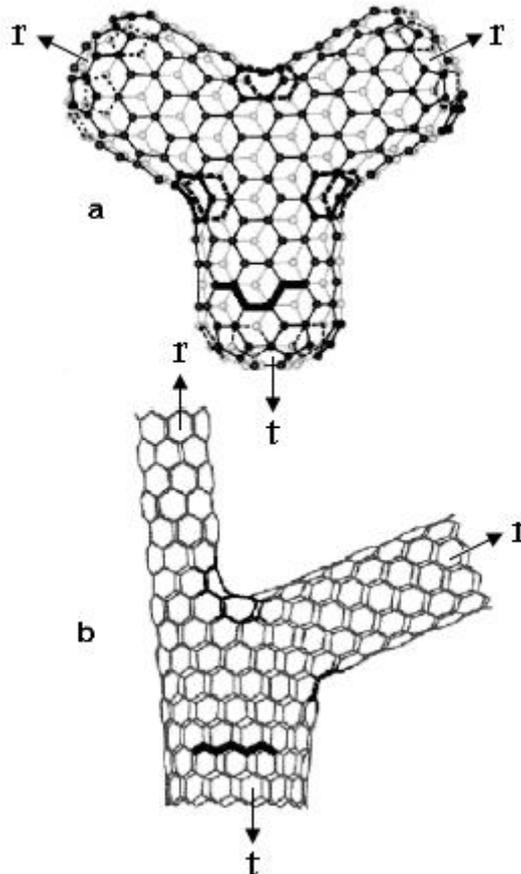
Fig. 1. Structural models of Y-junctions carbon nanotubes. Symmetric (a), armchair (b).
