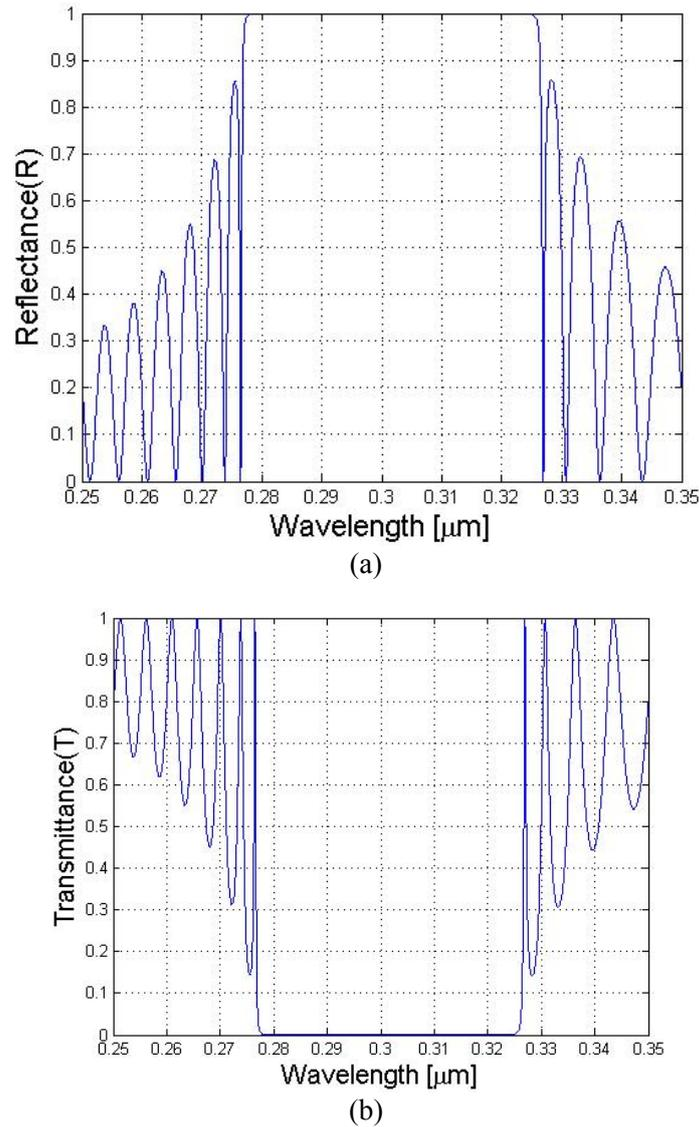
Fig. 2 (a) reflectance and (b) transmittance spectrum of the proposed filter.
