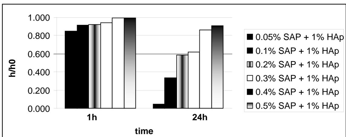
Fig.3. The ratios of sedimentation height ( $h$ ) to the initial suspension height ( $h_0$ ) of the suspensions
