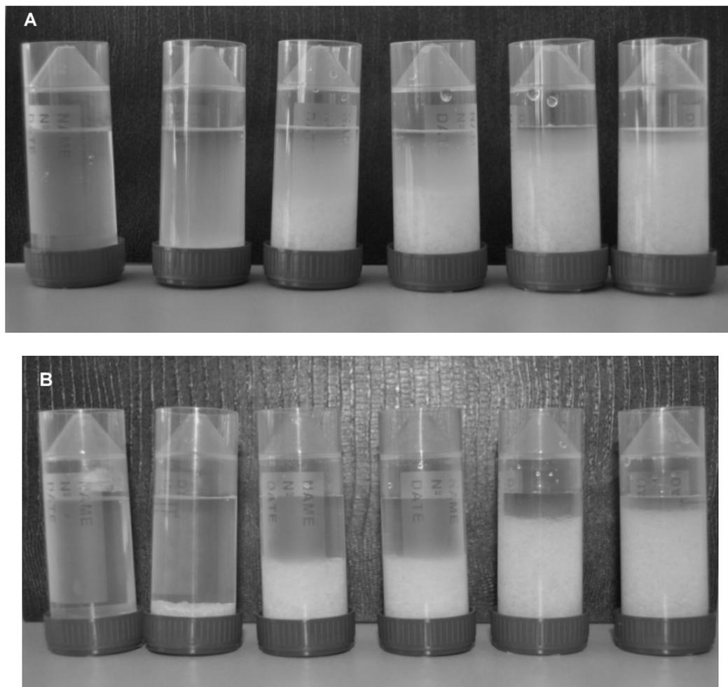
Fig. 4. Sedimentation behavior after (a) 1 h and (b) 24 h
