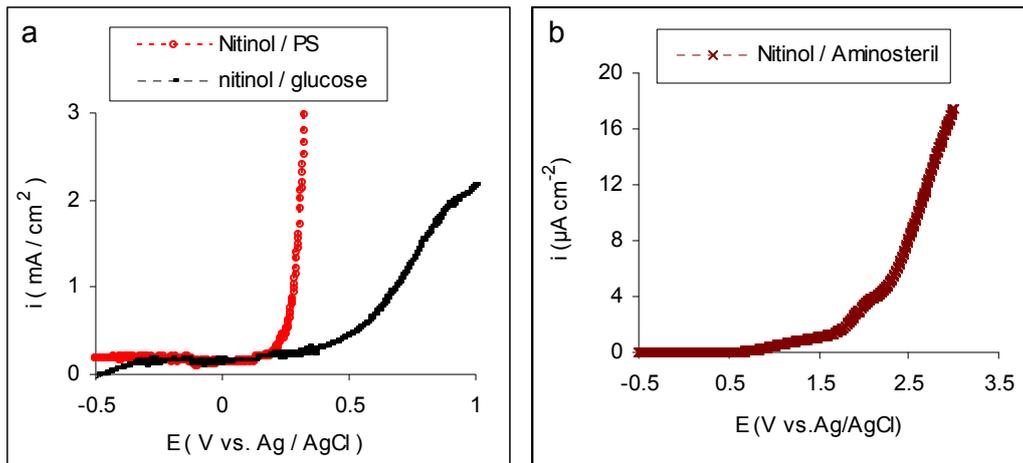
Fig. 1. Potentiodynamic curves of NiTi obtained in different artificial physiological media: a – physiological serum (PS) and glucose solutions; b – aminosteril solution
