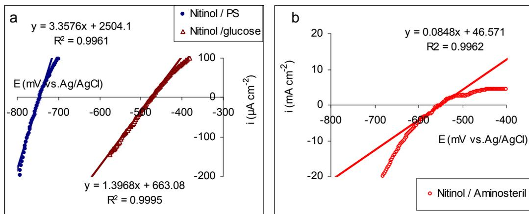
Fig. 3. Potentiodynamic curves near  $E_{\text{corr}}$  of NiTi obtained in different artificial physiological media: a – physiological serum (PS) and glucose solutions; b – aminosteril solution
