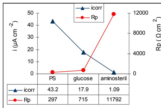
Fig. 4. The numerical values of corrosion currents and polarization resistances obtained for NiTi in different artificial physiological media
