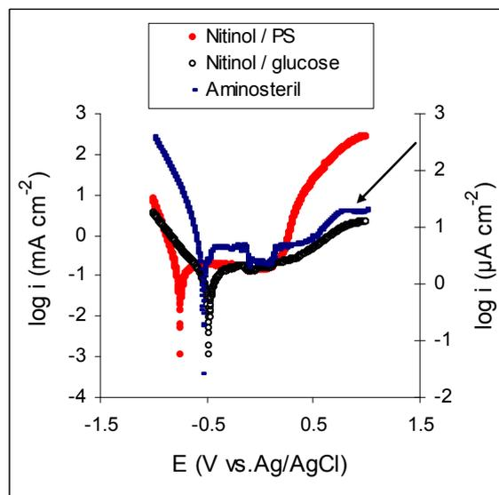
Fig. 2. Tafel diagram of NiTi corroded in various artificial physiological media
