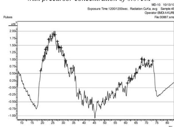
*Fig 1(i): XRD diffractogram for  $Fe_2O_3$  films with precursor concentration of 0.100M*
