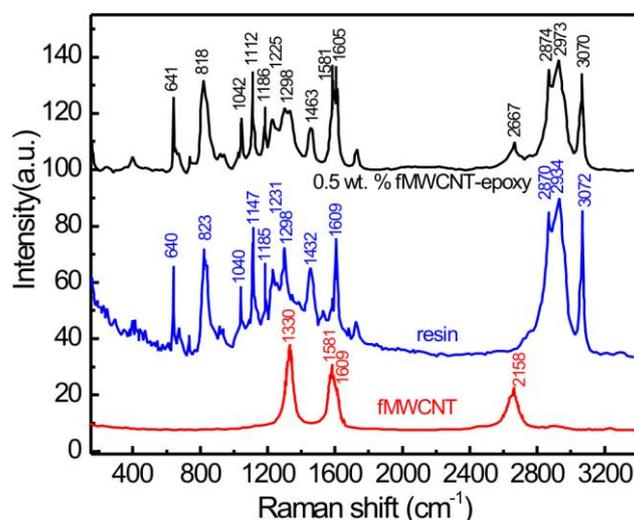
Fig. 1 Raman spectra of fMWCNT, epoxy resin and the 0.5 wt. % fMWCNT-epoxy composite.
