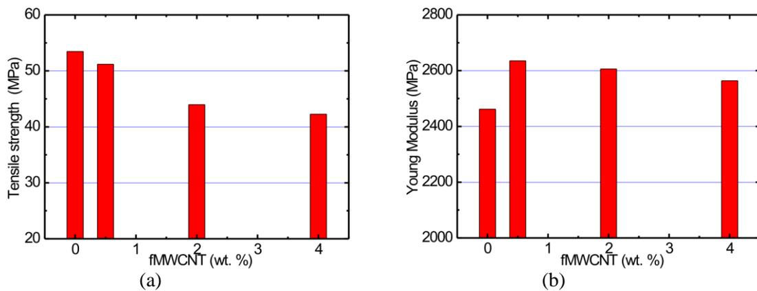
Fig. 5 (a) Tensile strength and (b) Young modulus at tensile stress at the breaking point.
