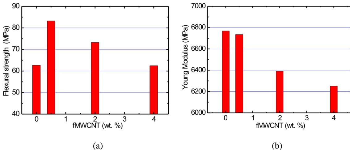
Fig. 3 (a) Flexural strength and (b) Young modulus at tensile stress for a transverse deflection of 6 mm.
