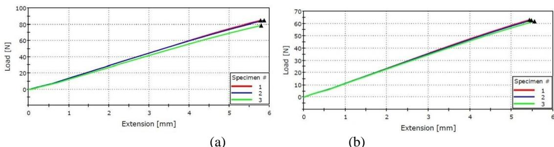
Fig. 6 Mechanical measurements for a deflection of 6 mm for fMWCNT-epoxy composites with fMWCNT mass concentration of (a) 0.5%, and (b) 4%
