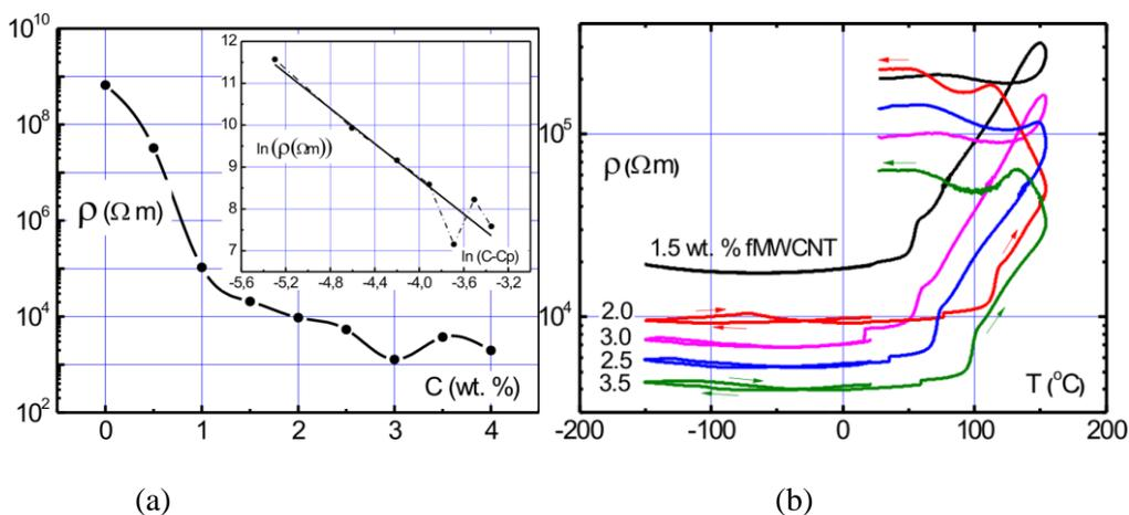
Fig. 14 (a) Dependence of the resistivity of epoxy composites on the fMWCNT concentration at room temperature. (b) Temperature dependence of the resistivity of fMWCNT-epoxy composites.
