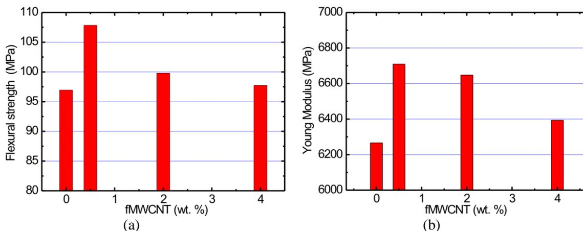
Fig. 4(a) Flexural strength and (b) Young modulus at tensile stress at the breaking point.
