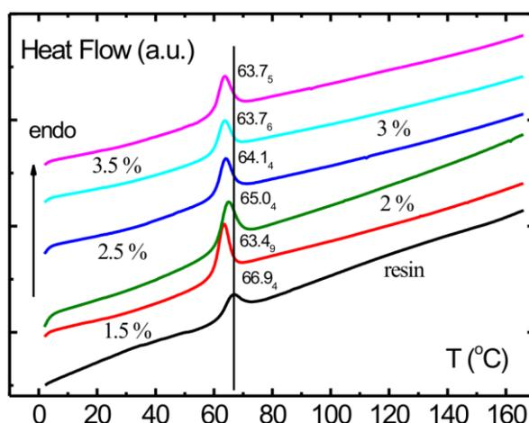
Fig. 2 DSC analyses of the epoxy resin and its composites with different fMWCNT mass contents.
