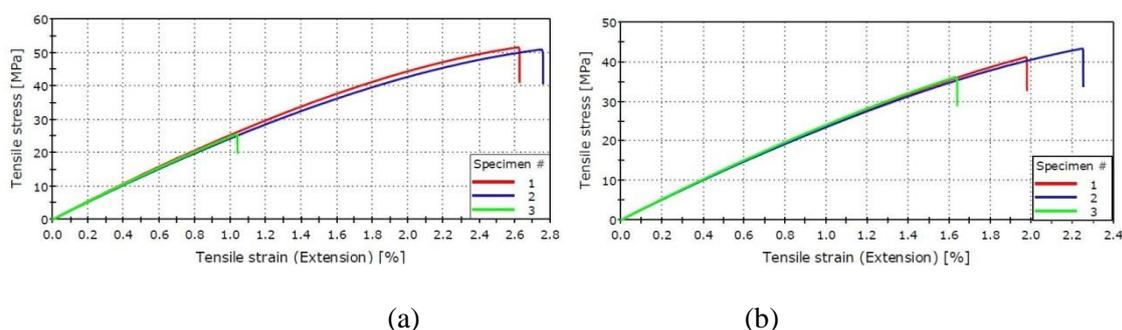
Fig. 8 Stress-strain curves at tensile stress forepoxy composites with (a) 0.5 wt. % fMWCNTs, and (b) 4 wt. % fMWCNTs
