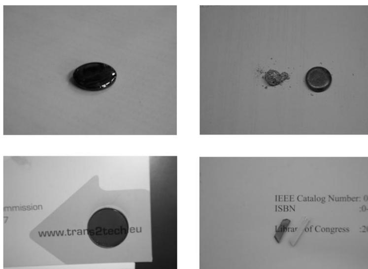
*Fig.3. Images of GLS samples with the same 70%Ga<sub>2</sub>S<sub>3</sub>/30% La<sub>2</sub>S<sub>3</sub> composition. Vitreous state corresponding to quenching from 1150 °C in Argon jet (up left); Glass after polishing (down left); Foam state (up right) is obtained after heating the bulk glass up to 900 °C and quenching in Argon flow. Piece of re-crystallized at 620 °C material compared to a transparent glass before heating (down right).*
