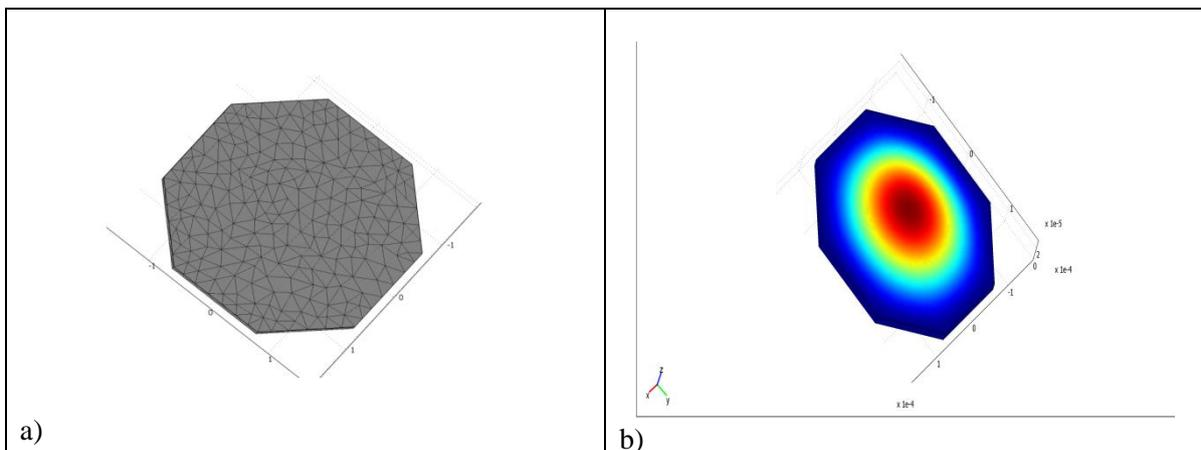
Fig. 1: (a),(b) The proposed octagonal diaphragm with a radius of 350  $\mu\text{m}$ .
