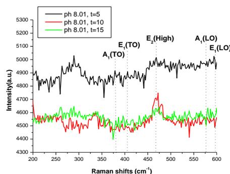
*Fig. 4. Raman Spectra of ZnO Nanoparticles prepared by Assisted Microwave Irradiations at pH 8.*
