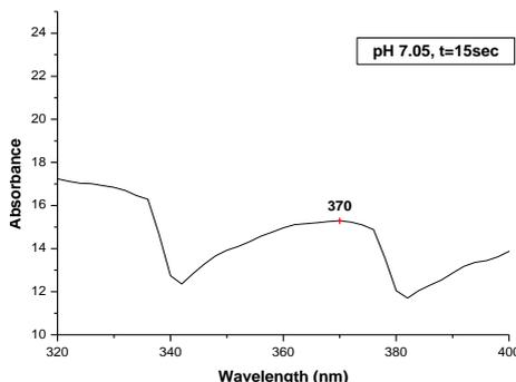
Fig. 1. UV-Visible absorption spectrum for microwave assisted ZnO nanoparticles at pH 7.0 for 15 sec.
