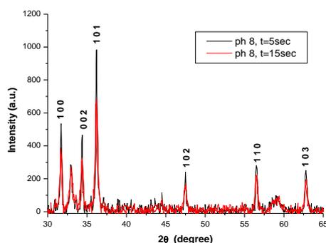
Fig. 3. XRD Pattern of Sample with pH 8 by Assisted Microwave Radiations for time 5sec and 15sec.
