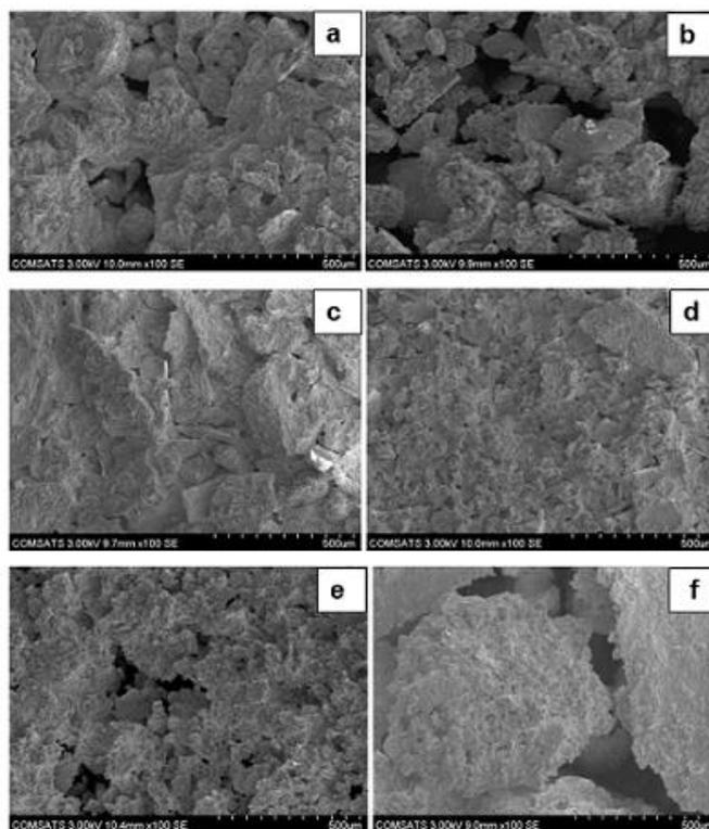
Fig. 5. SEM Images of ZnO Nanoparticles at pH 6.0 Assisted by Microwave Radiations for (a) 5sec and (b) 15 sec, at pH 7.0 (c) 5 sec and (d) 15 sec. at pH 8.0 (e) 5 sec and (f) 15 sec.
