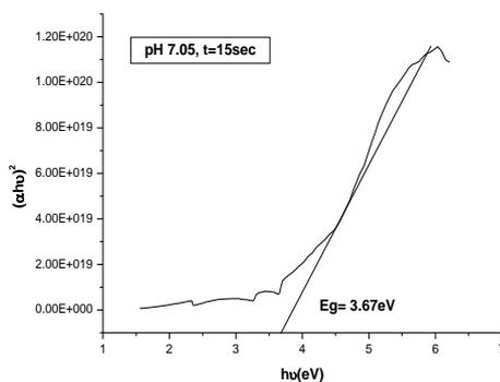
Fig. 2. Bndgap of CuS nanoparticles at pH 7.0 Assisted by Microwave Radiations for 15sec.
