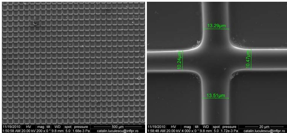
Fig. 3. SEM images of a 60x60 lines polymerized SIM 3 sample, Photoinitiator = IRG 369, Distance between lines = 50  $\mu\text{m}$ , Scanning velocity = 1 mm/s, Laser incident power = 15 mW.
