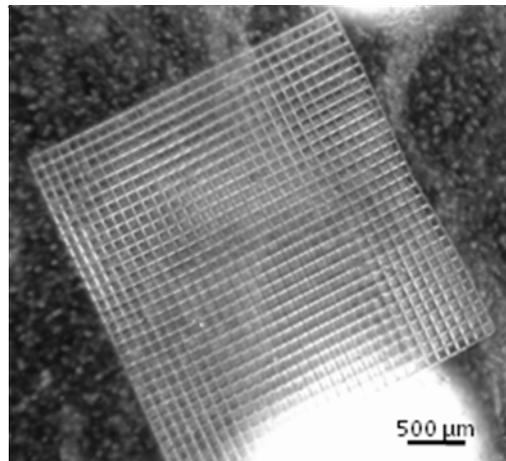
*Fig. 5. Optical image of a free-standing structure 3x3 mm<sup>2</sup> generated by the mixture SIM 3 and UDA. Spacing between lines 100  $\mu\text{m}$ ; Scanning velocity = 1 mm/s, Laser incident power = 15 mW.*
