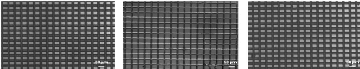
Fig. 2. Optical microscopy images of polymerized (a) SIM 3 (b) UDA (c) SIM 3 +UDA, Photoinitiator = Irgacure 369, Distance between lines = 50  $\mu\text{m}$ , (a) Laser incident power = 15 mW, Scanning velocity = 1 mm/s; (b) Laser incident power = 10 mW, Scanning velocity = 3 mm/s; (c) Laser incident power = 15 mW, Scanning velocity = 1 mm/s.
