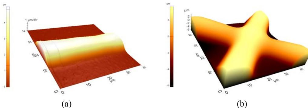
Fig. 4. AFM images of (a) a line of polymerized SIM 3; (b) a crossing of a polymerized SIM 3; Scanning velocity = 1 mm/s, Laser incident power = 15 mW.
