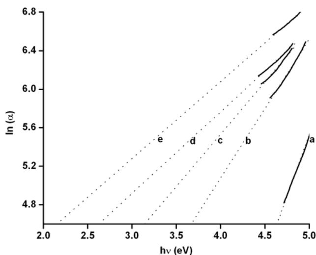
Fig. 5 Plots of  $\ln(\alpha)$  versus  $h\nu$  for (a) pure PVP and PVP-Ag nanocomposites (b) without exposure; with exposure to ultraviolet radiations for (c) 30; (d) 90 and (e) 180 minutes.
