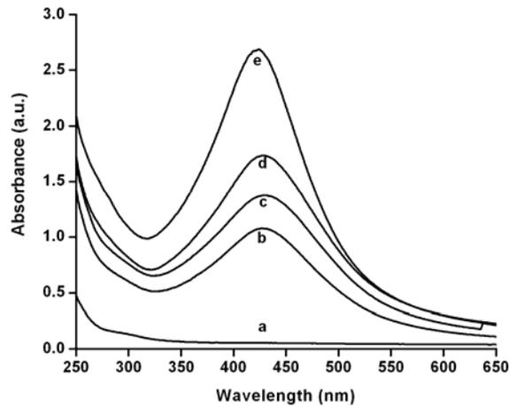
Fig. 3 UV-Visible absorption spectra for (a) pure PVP and PVP-Ag nanocomposites (b) without exposure; with exposure to ultraviolet radiations for (c) 30; (d) 90 and (e) 180 minutes.
