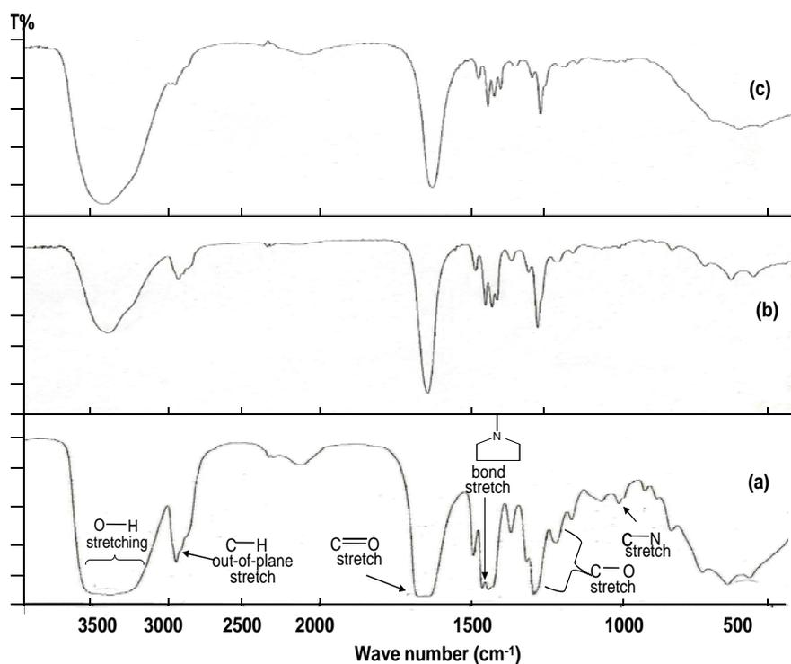
Fig. 7 FTIR spectrum for (a) Pure PVP; PVP-Ag nanocomposite (b) without exposure and (c) for 180 minutes exposure to ultraviolet radiation.
