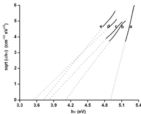
Fig. 4 Plots of  $\text{sqrt}(\alpha h\nu)$  versus  $h\nu$  for (a) pure PVP and PVP-Ag nanocomposites (b) without exposure; with exposure to ultraviolet radiations for (c) 30; (d) 90 and (e) 180 minutes.
