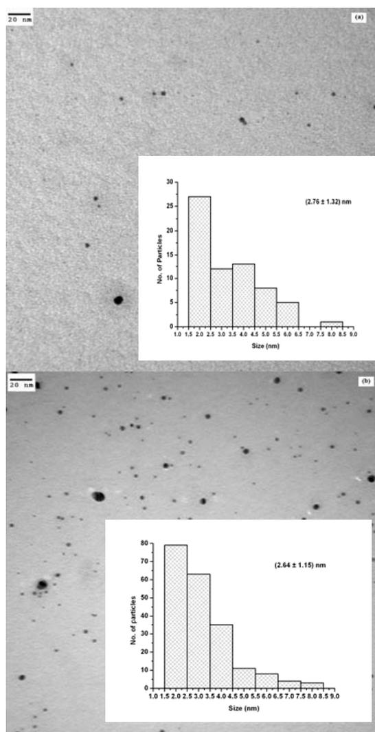
Fig. 2 Transmission electron micrographs with particle size distribution of embedded Ag nanoparticles in PVP (a) before exposure to UV radiation; (b) after exposure to UV radiation for 180 minutes.
