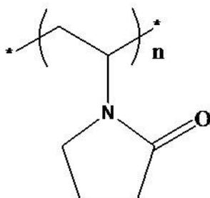
Fig. 1 Monomer structure of PVP.
