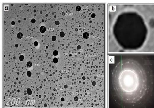
Fig. 2. HR-TEM micrographs of CuO NPs biosynthesized using *A. fumigatus* preformed biomass from  $\text{Cu}(\text{NO}_3)_2 \cdot 3\text{H}_2\text{O}$ . (a) Showing spherical uniformly distributed NPs (b) Outlines of single magnified NP and (c) SAED pattern recorded for one NP.
