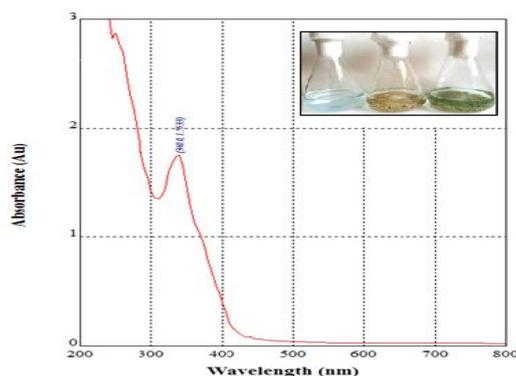
Fig. 1. UV-Vis absorption spectrum of CuO NPs formed using biomass of *A. fumigates*. Inset shows color change after incubating the biomass in 1mM copper nitrate (Right), in comparison with the biomass in double distilled water as positive (Middle) and copper nitrate alone as negative (Left) controls.
