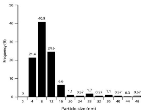
Fig. 3. Particle size distribution of CuO NPs from TEM analysis.
