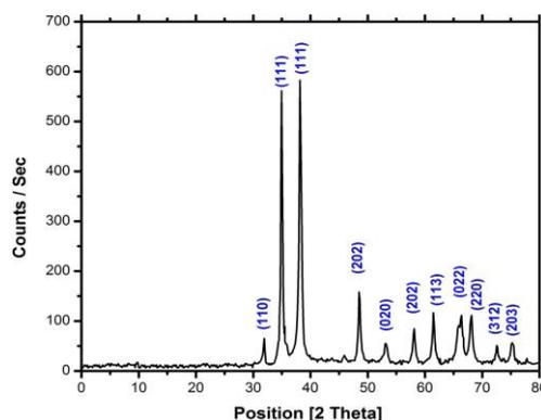
Fig. 4. XRD pattern of CuO NPs biosynthesized using biomass of *A. fumigatus*.
