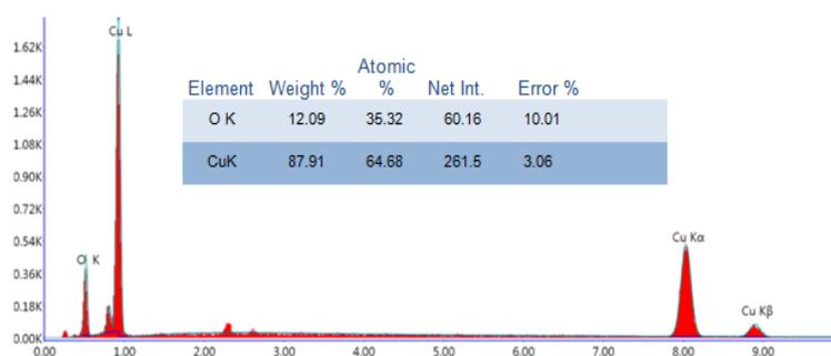
Fig. 7. EDX pattern of CuO NPs from *A. fumigatus* biomass
