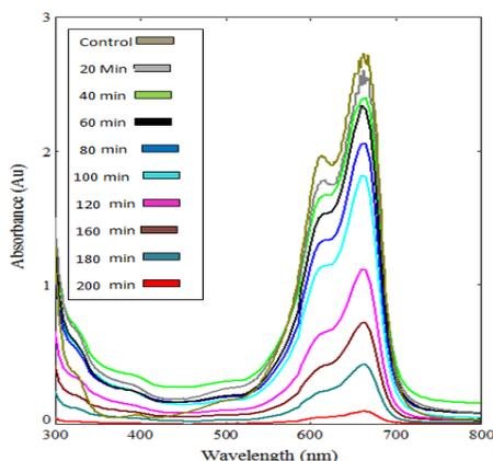
Fig. 9. UV-Vis spectra for photocatalytic degradation of MB by CuO NPs biosynthesized using *A. fumigatus*.
