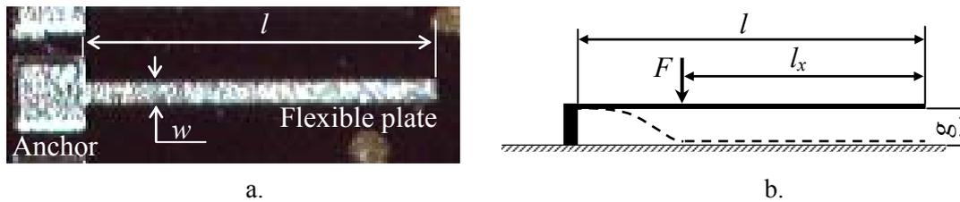
Fig.2. Microcantilever for experimental investigations (a), and an instantaneous position of the load on microcantilever (b)
