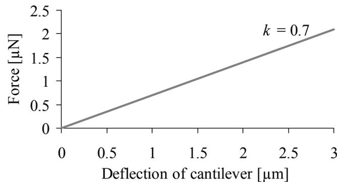
Fig.3. Force versus deflection of a microcantilever (the force is applied at the free-end of sample)
