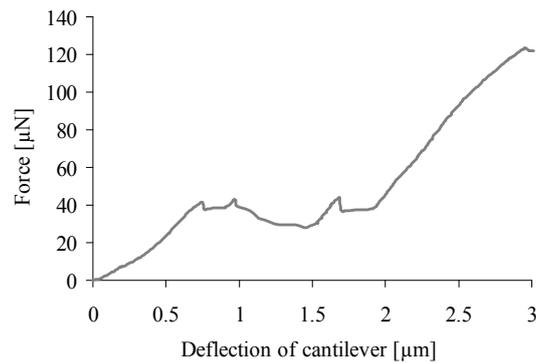
Fig.4. Nonlinear dependence between force and deflection of a microcantilever (the force is applied close to the beam anchor)
