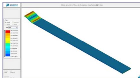
Fig. 6. Stress distribution in the investigated microcantilever subjected to plastic deformations
