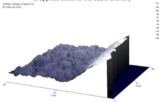
Fig.5. Inelastic deformation of a microcantilever when the force is applied close to the beam anchor.
