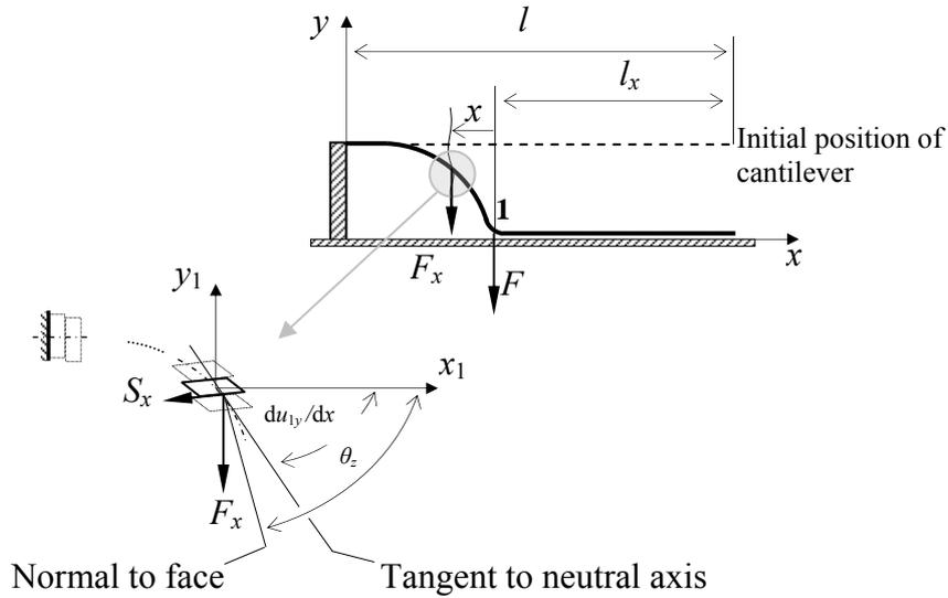
Fig.1. Microcantilever under bending and shearing deformations.
