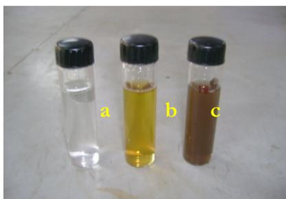
Fig 1. Optical photograph of (a) 1 mM  $\text{AgNO}_3$  solution (b) Leaf extract (c) Leaf extract +  $\text{AgNO}_3$  after 48 h of reaction
