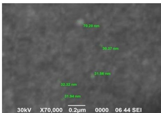
Fig 4. SEM image of synthesized Ag nanoparticles
