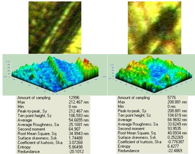
Fig. 6. Ti6Al4V surface microgeometry and tribological parameters measured using NTEGRA Atomic Force Microscopy
