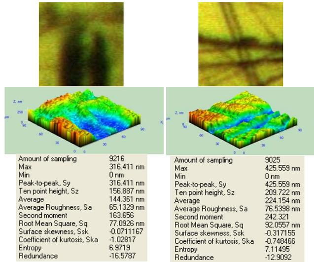
Fig. 5. Stainless steel surface microgeometry and tribological parameters measured using NTEGRA Atomic Force Microscopy
