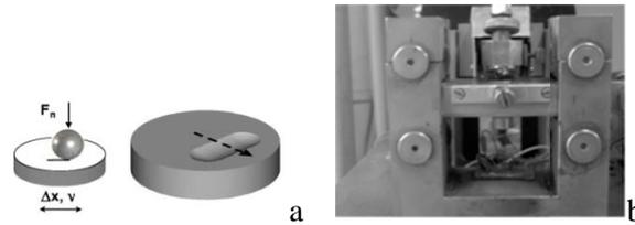
Fig. 3. Coated disks were tested articulating against a ball (polished surface) on top of a disk (a) and experimental device (b).
