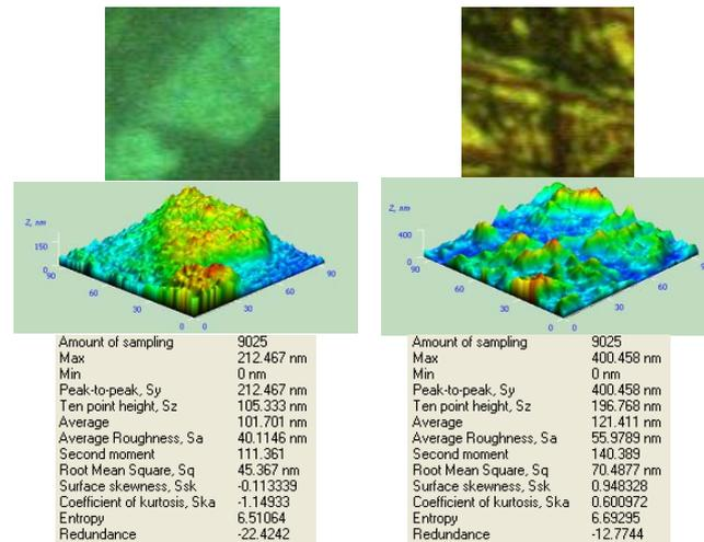
Fig. 7. CoCr surface microgeometry and tribological parameters measured using NTEGRA Atomic Force Microscopy.
