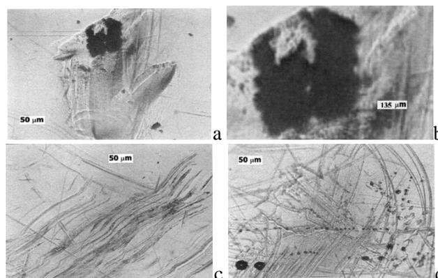
Fig. 4. Images obtained with AFM. Scratching (a), embedded wear particle (b) micro-cutting (c) and corrosion fretting (d) of femoral head.
