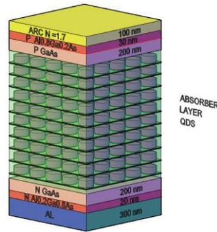
Fig. 2. The schematic of the proposed solar cell and thicknesses of different layers. Details of the structure are expressed in the Table 1.
