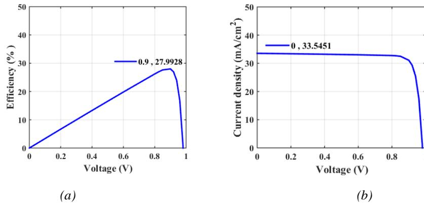
Fig. 7. (a) Efficiency-voltage curve and (b) current density-voltage curve of the proposed solar cell
