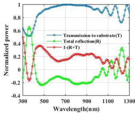
Fig. 6. Transmission, total reflection and absorption of proposed structure.
