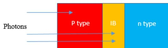
Fig. 1. General structure of an intermediate-band solar cell.
