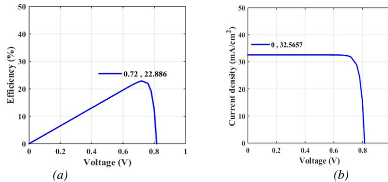
Fig. 3. (a) Efficiency-voltage curve and (b) current density-voltage curve of the reference solar cell
