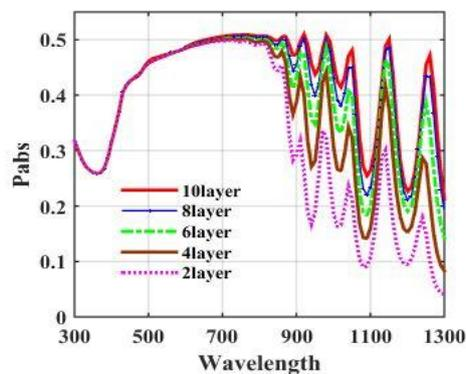
Fig. 5. Wavelength-absorption curve for different number of cylindrical quantum dot layers.
