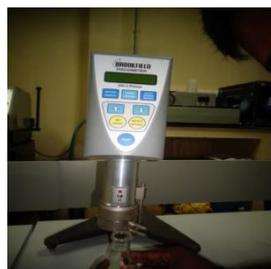
Fig.3. Brookfield Viscometer
