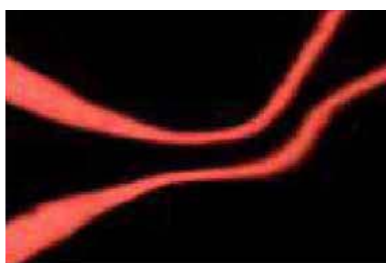
Fig.5(a) Double flow switching from inlets B, D to outlets 1 and 2, the voltage difference between B and D is 600V
