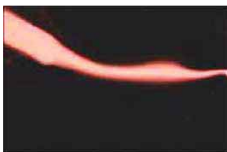
Fig.4(c) Single flow switching from inlet B to outlet 3 with applied DC voltage, the voltage difference between B and outlet 3 is 800V
