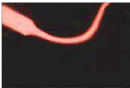
Fig.4(a) Single flow switching from inlet B to outlet 1 with applied DC voltage, the voltage difference between B and outlet 1 is 800V
