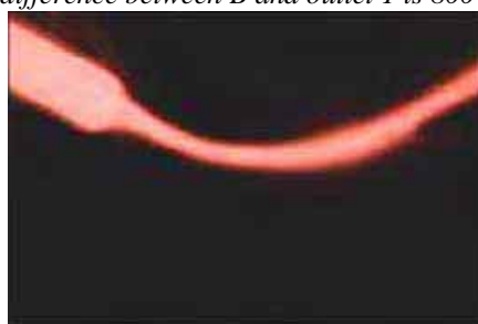
Fig.4(b) Single flow switching from inlet B to outlet 2 with applied DC voltage, the voltage difference between B and outlet 2 is 800V
