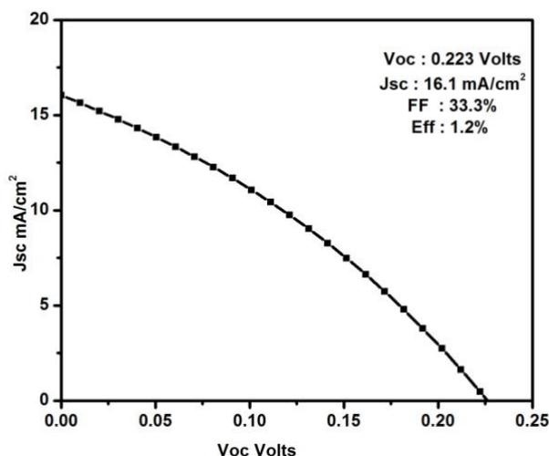
Fig. 5 Solar cell photo conversion efficiency
