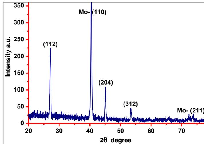
Fig. 1 X-ray diffraction of CZTS/Mo/SLG thin film layers
